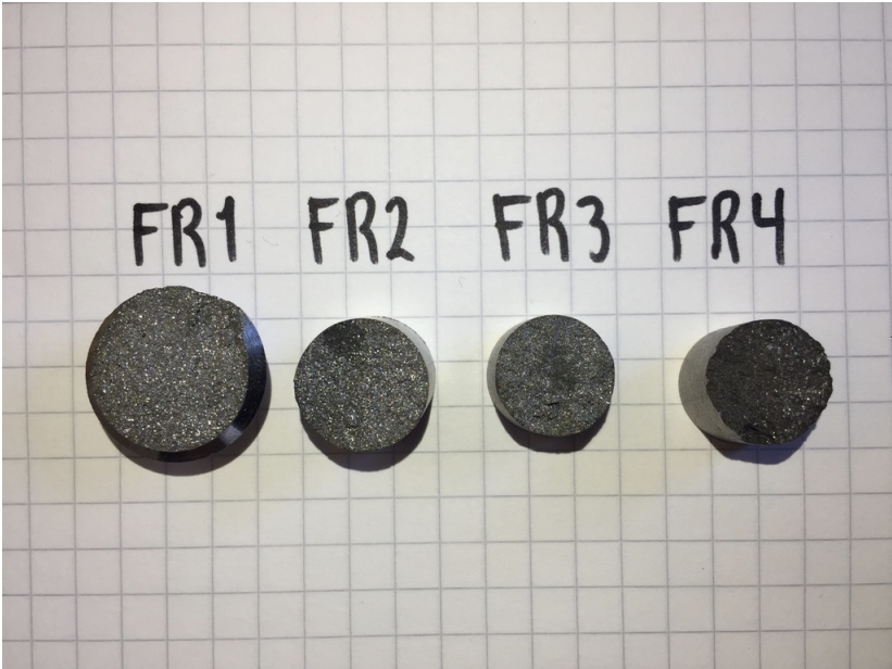
Figure 4.2: Fracture surface of the 4 cut tensile bars
