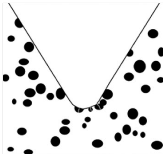
Figure 3.1: Schematic illustration of notch sensitivity in ductile iron (Wallin, 2014)
