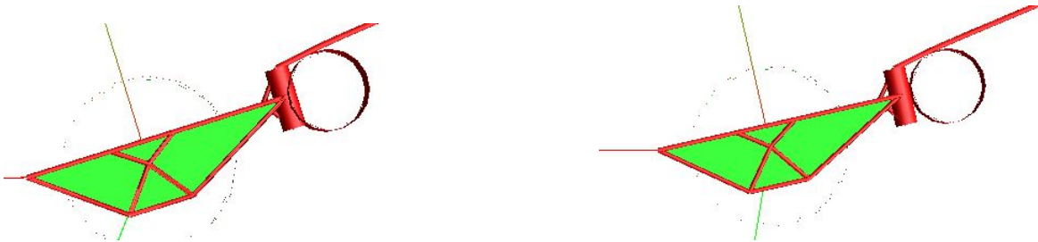
Figure 6.19 Clump weight with penetration due to low contact stiffness Figure 6.20 Clump weight with no penetration due to average stiffness
