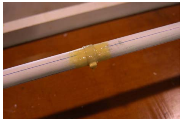
Figure 2.14 Riser instrumentation: a) strain gauge and b) accelerometer (Braaten and Lie, 2005)
