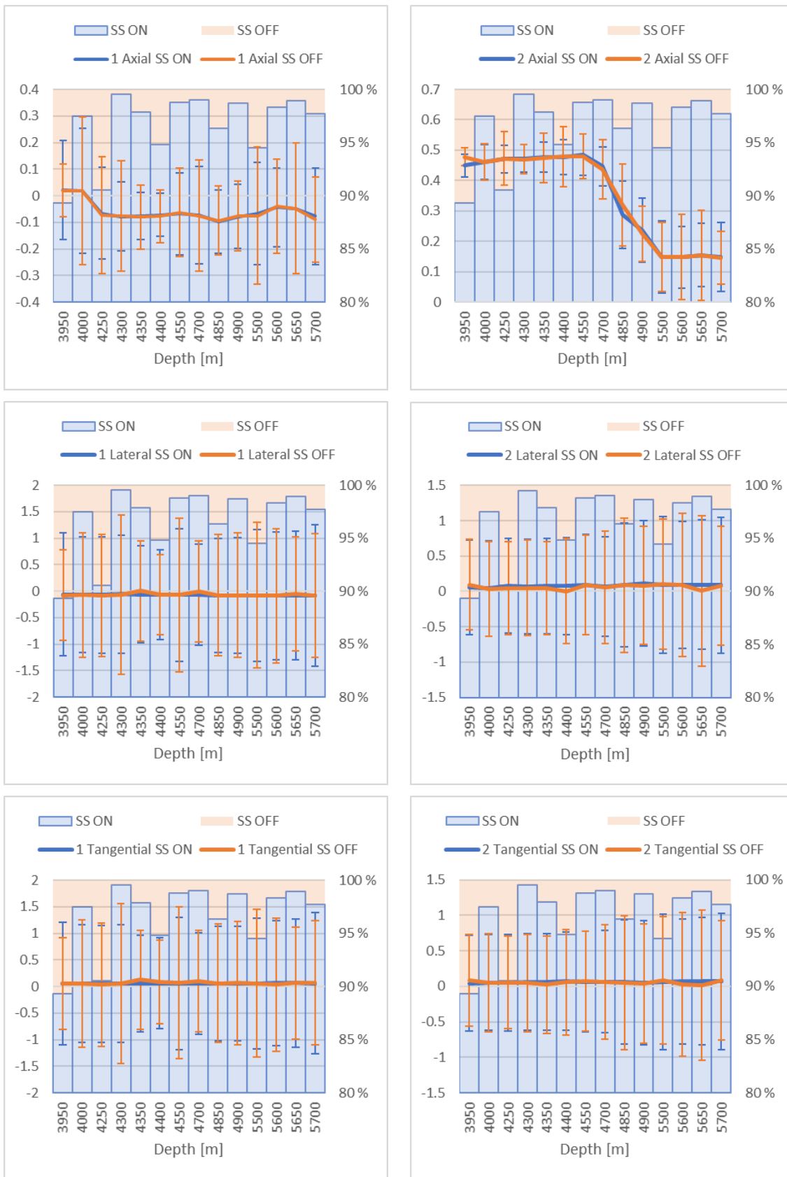
Figure 4.64: Effects of SoftSpeed on drilling vibrations in well 1.4
