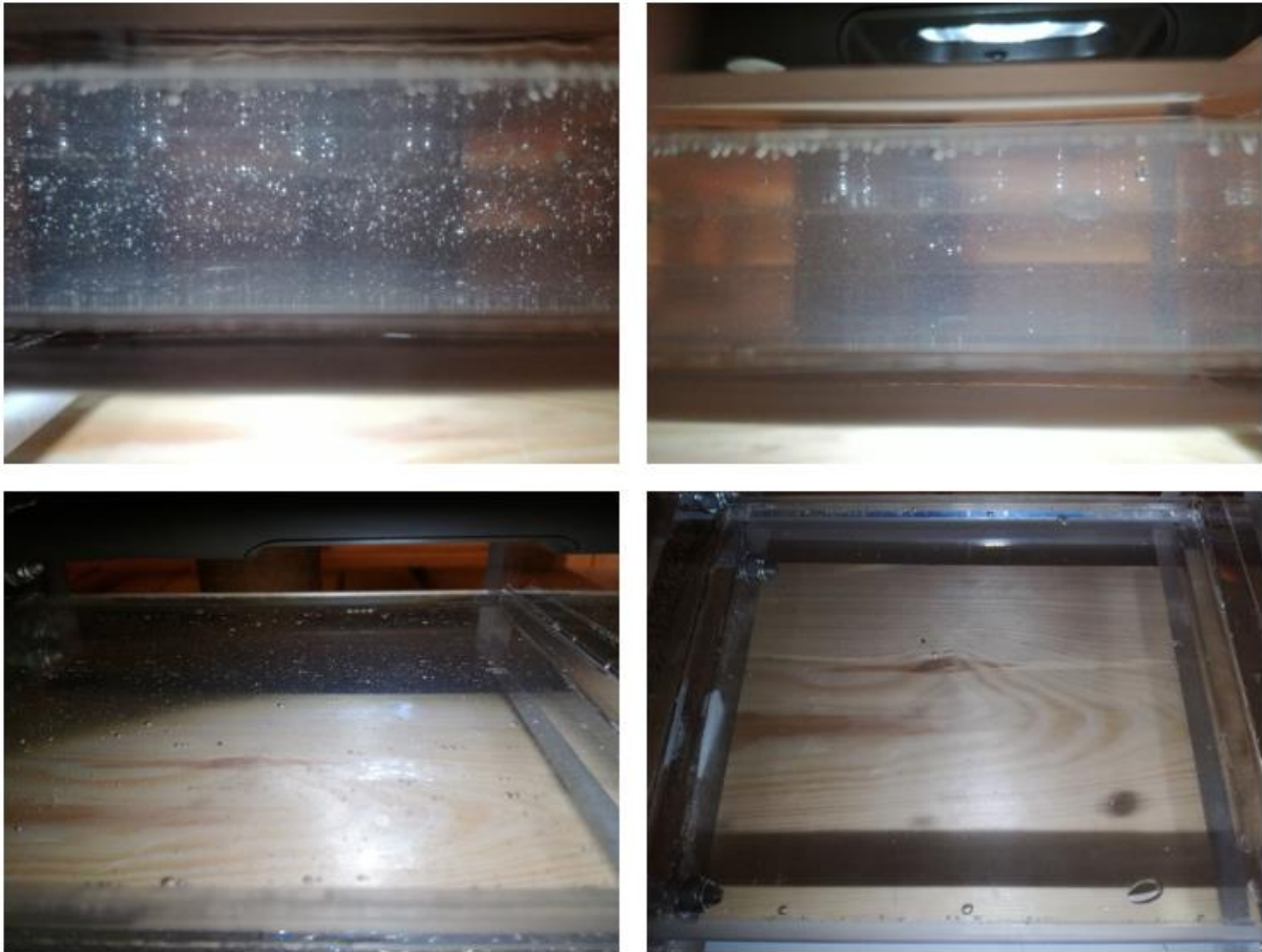
Figure 5.22: Carbopol in flow channel (left). Condition after leaving it static in the channel for 24 hours (right).
