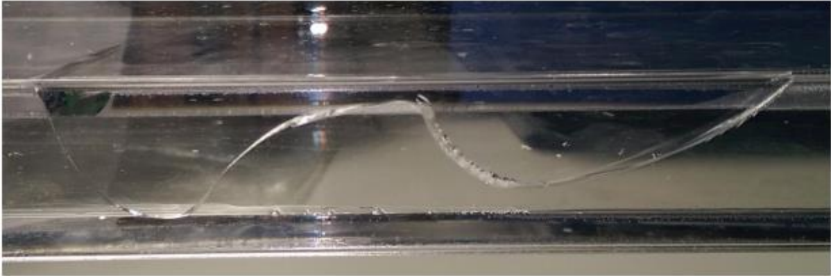
Figure 5.11: Second crack in acrylic duct.
