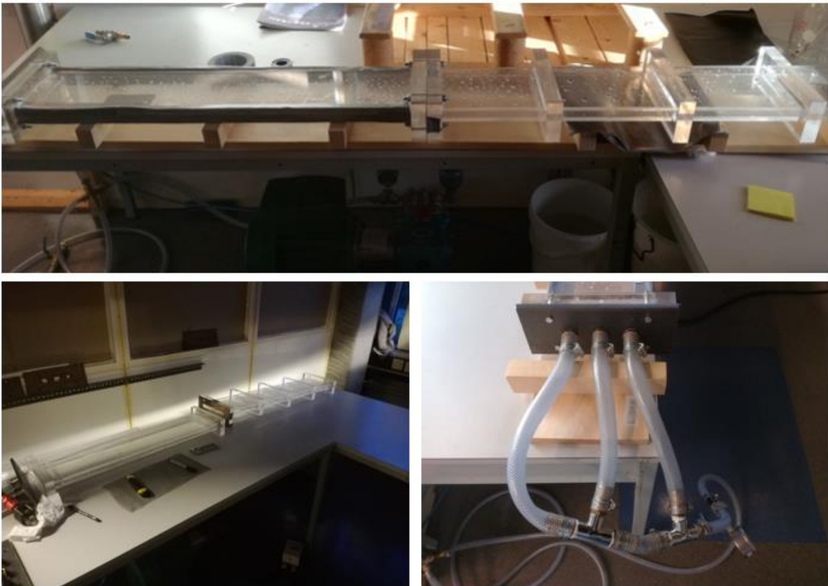
Figure 5.14: Final flow channel setup used for PIV experiments.
