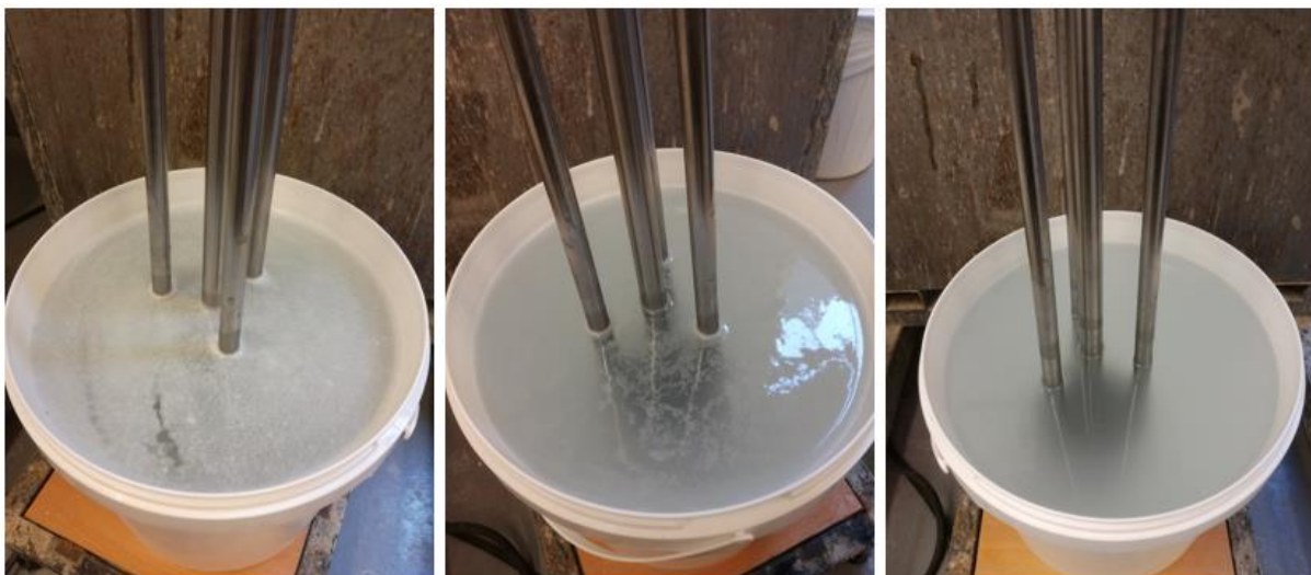
Figure 5.21: Carbopol dispersed in water after 30 min (left). Condition of the solution after 7 hours agitation (middle) and solution left static for 12 hours (right) before neutralization.
