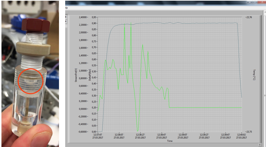
Figur 31: Hidden air bubble. The scapegoat was detected because it was believed that the problem had to do with the electrode somehow. The graph illustrates how stability suddenly appeared (green line) when the electrode chamber was flicked vigorously several times. In the first section the streaming potential is rapidly changing with several volts in magnitude, even the pressure is stabilised. It is credible that this bubble was blocking coherent brine between the electrode chamber and the brine from the rest of the system.
