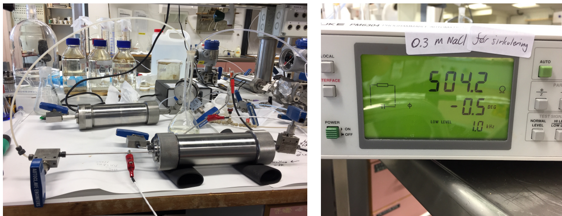
Figur 26: Resistance measurement. Brine is injected through the core and wasted until the resistance remains constant. Thus, the core is fully saturated with one distinct brine.
