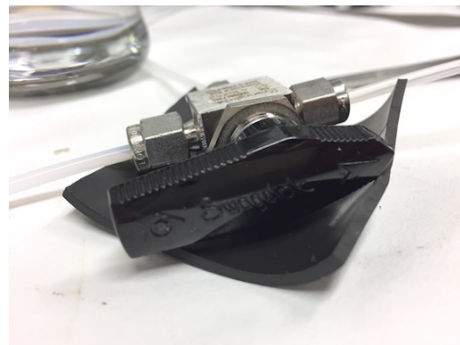
Figur 18: Isolation of metallic valves. All valves and other metallic parts that has any connection to the brine must be prescind from any sources that may disturb the measurements. This metallic valve was separated from the table with a clipped rubber sleeve.
