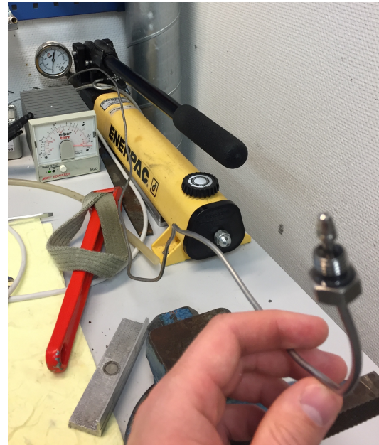
Figur 15: Manual hydraulic pump to generate a confining pressure around the core in the core holder.
