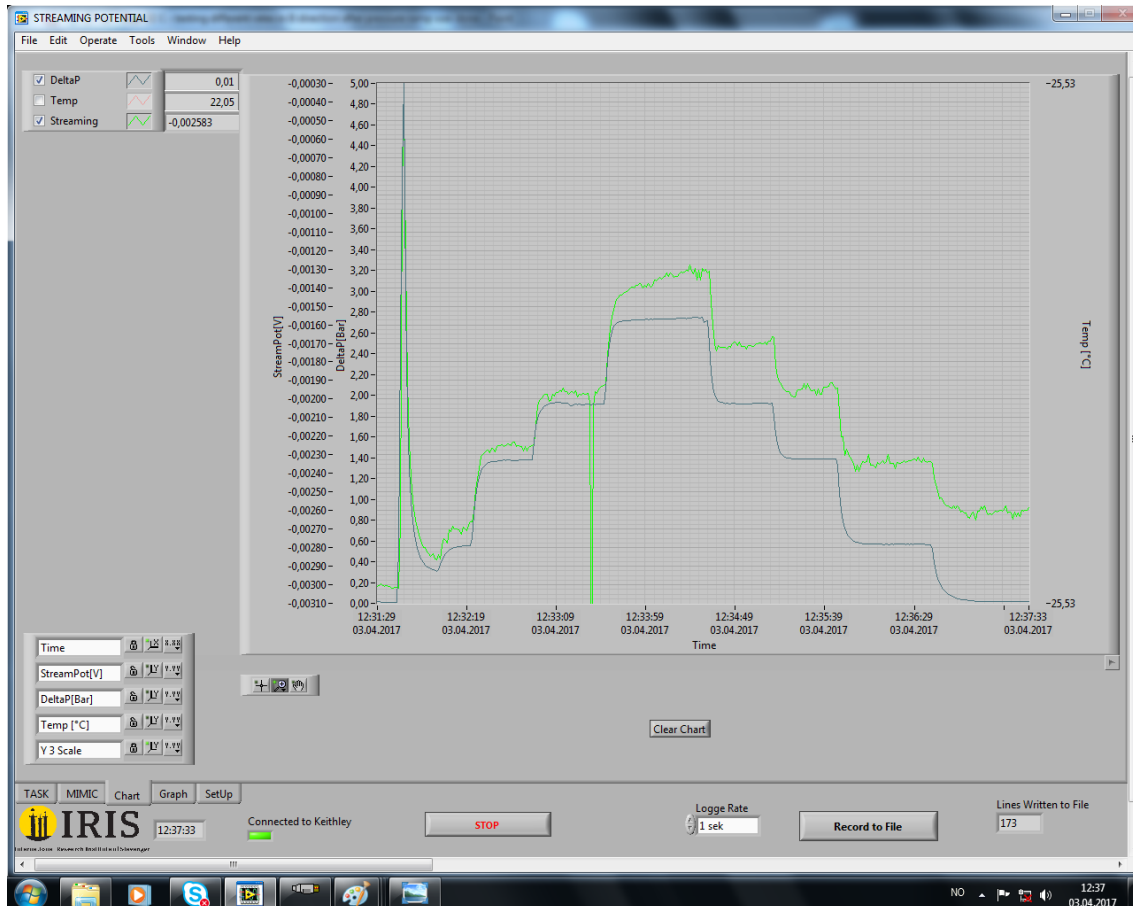
Figur 28: Screenshot from the laboratory computer. Pressure is increased and decreased stepwise. The streaming potential does not have the same value within the two distinct pressures due to variation in static voltage.
