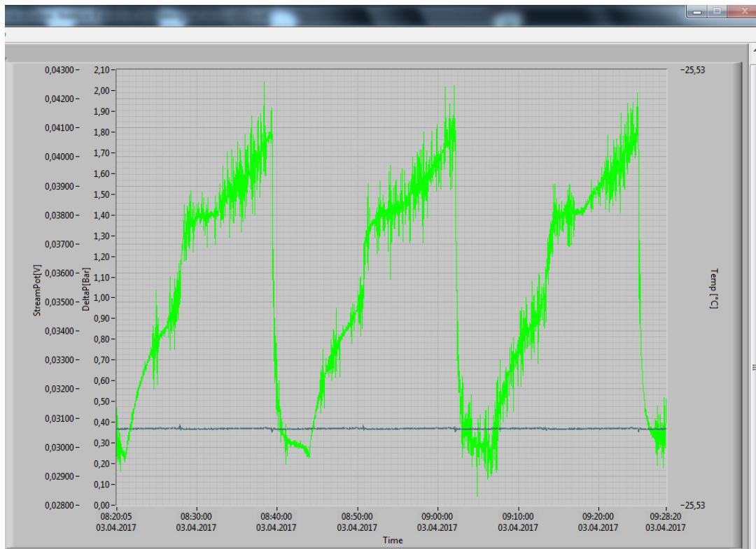
Figur 33: Pump disturbance. If the brine is flooded directly from the pump into the core, a parallel circuit is present.
