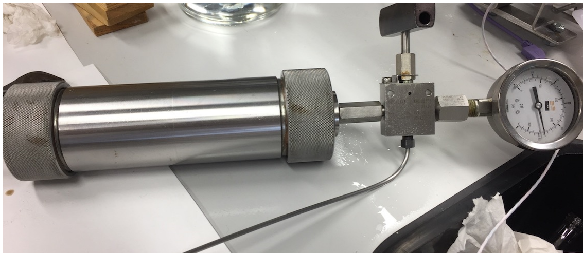
Figur 16: Confining pressure. Cylinder filled with compressed nitrogen in order to maintain confining pressure.
