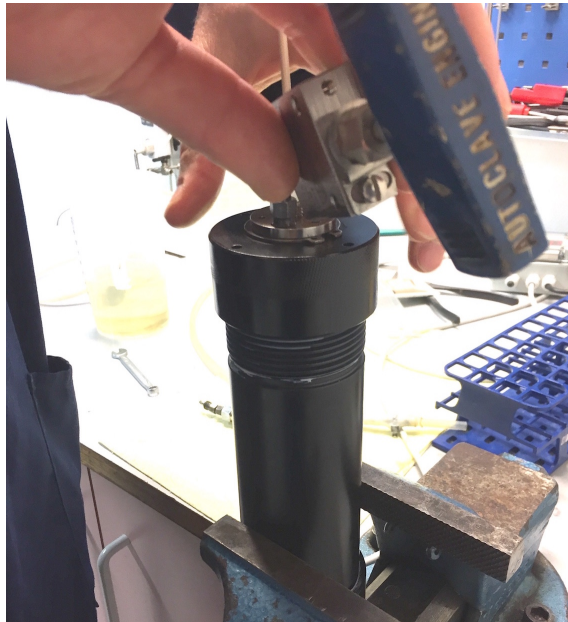
Figur 14: Assemble the core holder. The core was placed in the rubber sleeve and connected to the peak valves, it was tightly confined with synthetic oil.
