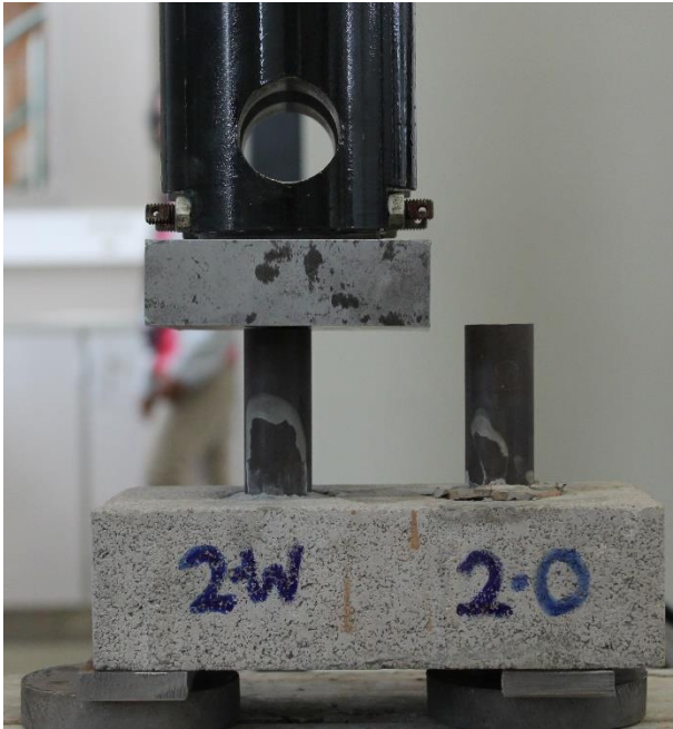
Figure 4.63: Setup for the shear bond strength test of the FCC specimens.
