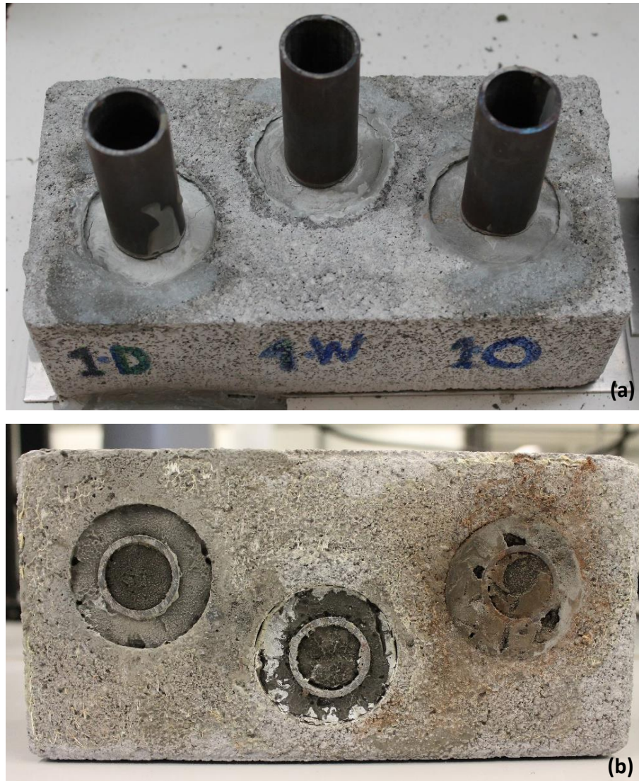
Figure 4.60: The set cement in a dry well, well with WBM and well with OBM, from left to right. (a) The top of the specimens, and (b) the bottom of the same specimens.
