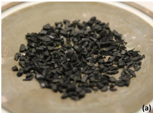
Figure 4.15: Cut O-rings (a) before acid treatment and (b) after acid treatment.
