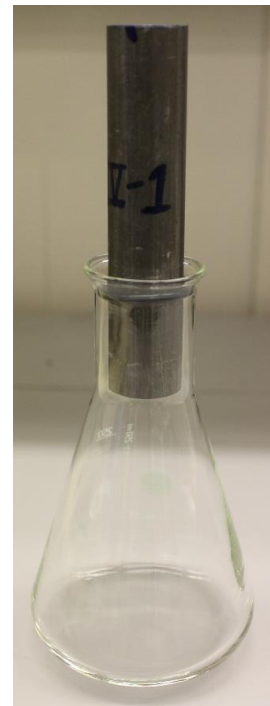
Figure 4.37: Setup for leakage test of CC-III.
