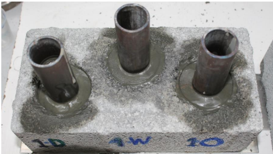
Cement poured between formation wall and casing (FCC-1)
