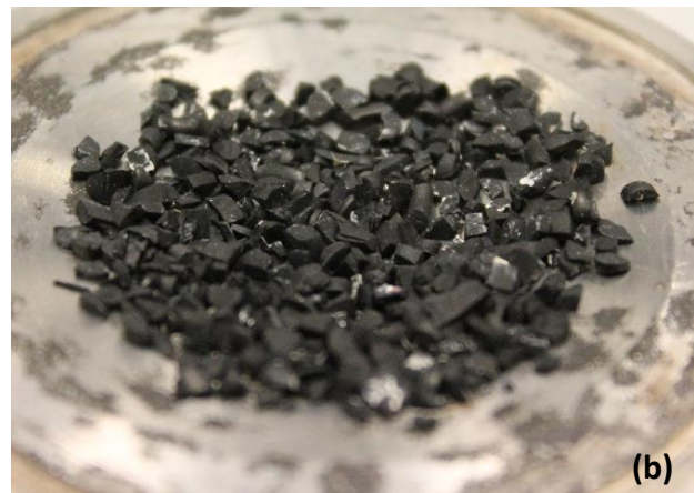
Figure 4.15: Cut O-rings (a) before acid treatment and (b) after acid treatment.
