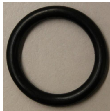
Figure 4.14: O-ring before it was cut.
