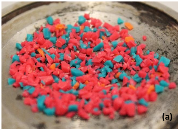
Figure 4.19: Cut silicone rubber (a) before and (b) after acid treatment.
