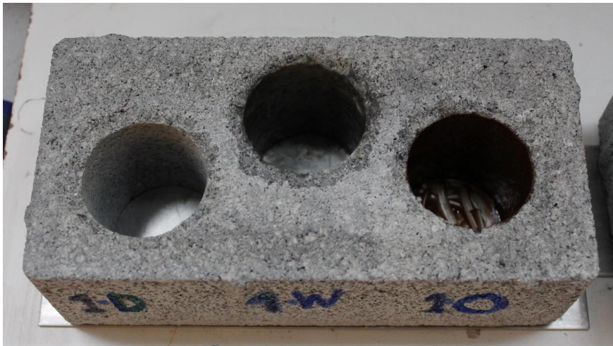
Mud applied on the borehole wall (FCC-1)
