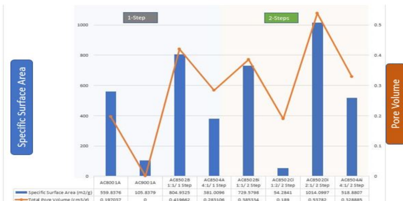
FIGURE 4.15: Effect of Temperature and Number of steps on Surface area and Pore volume
