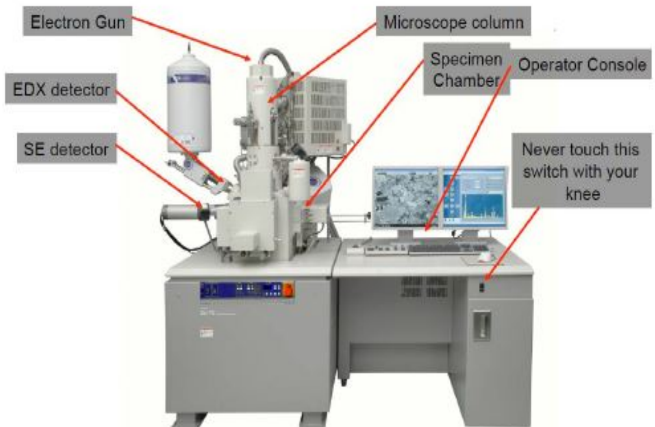
FIGURE 2.28: Scanning Electron Microscope [11]
