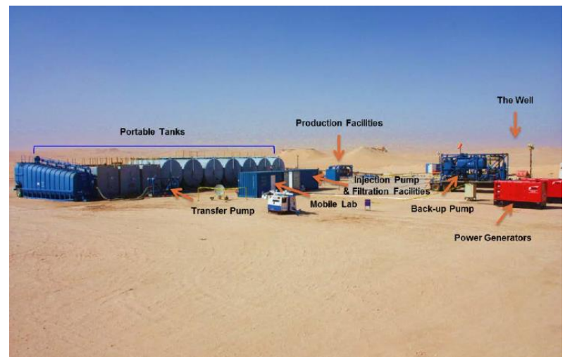
Figure 3.5: (a) Relative location of selected wells for SmartWater Flood field tests, (b) Overall field preparation and logistics at the well site.
