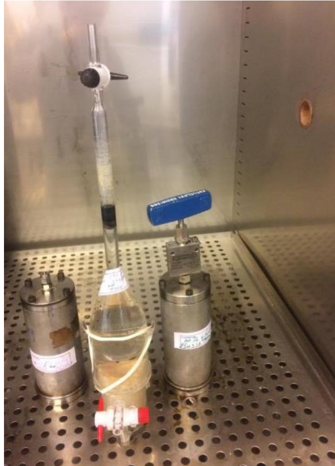
Figure 5.3: (middle) spontaneous imbibition SK-100; aging of SK-10 and SK-0 (left and right)
