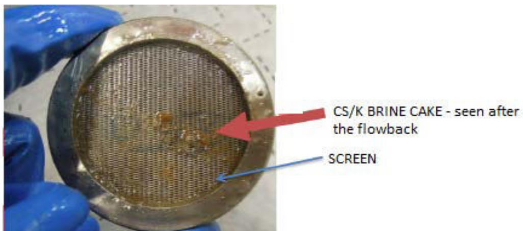
Figure 19 Mesh Screen and Cs/K brine cake after flowback
