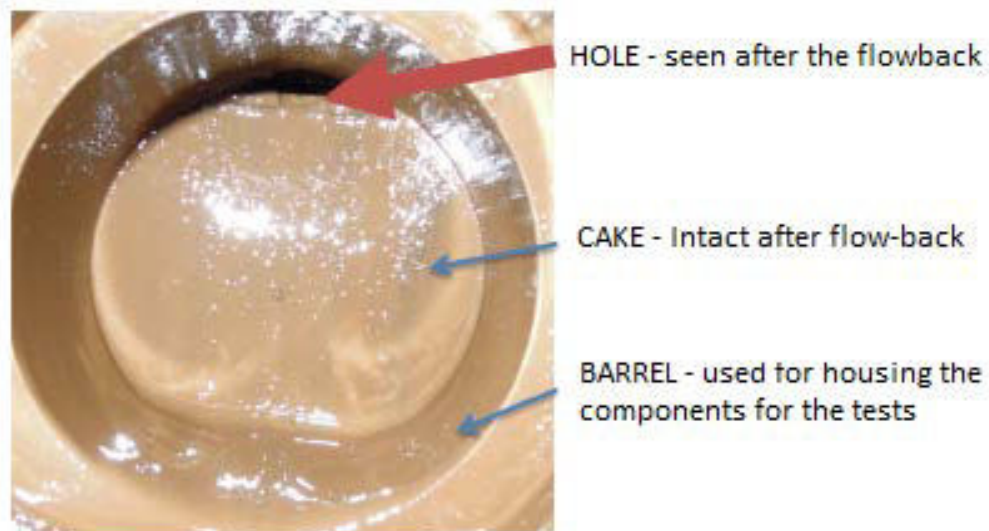
Figure 18 WARP OBM filter cake after flowback
