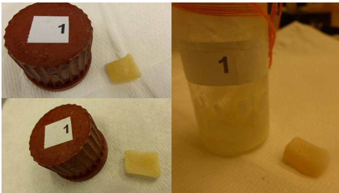
Figure 4-30: 5STY specimens after 24 hours in experiments with temperature 40°C, 60°C and 80°C
