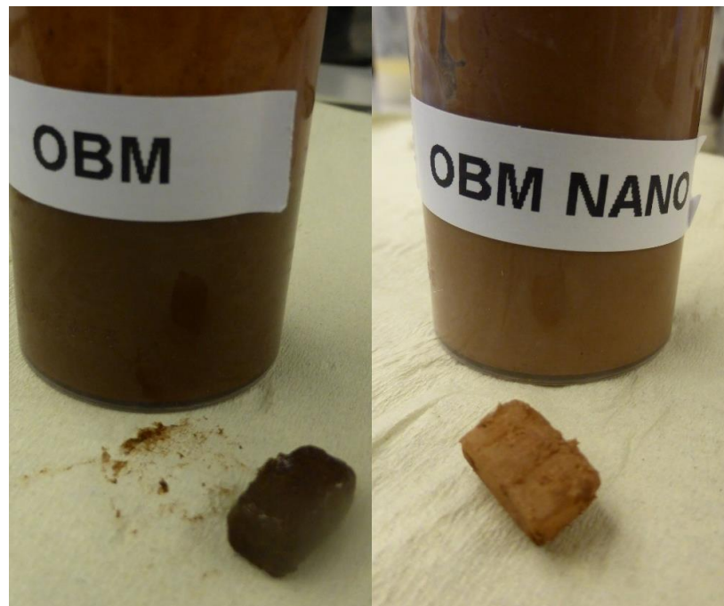
Figure 4-31: 5STY after 24 hours testing in OBM and OBM with TiO 2 nanoparticles solution
