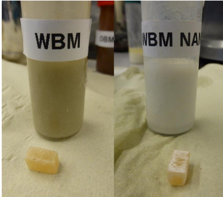
Figure 4-32: 5STY after 24 hours testing in WBM and WBM with TiO 2 nanoparticles solution
