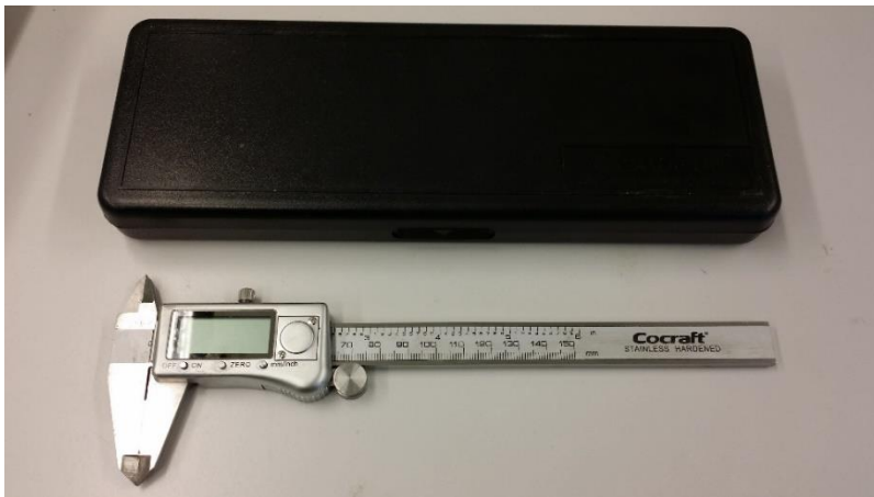
Figure 3-9: Digital Vernier caliper used for dimensional measurement
