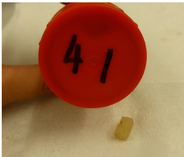
Figure 4-33: 41ACN in pure OBM after 24 hours
