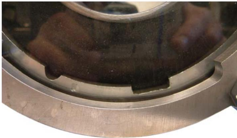
Figure 2-4: A picture showing the swelling rubber forming a pressure seal with a variety of geometry shaped containers (groves and rectangular cut out) [2]
