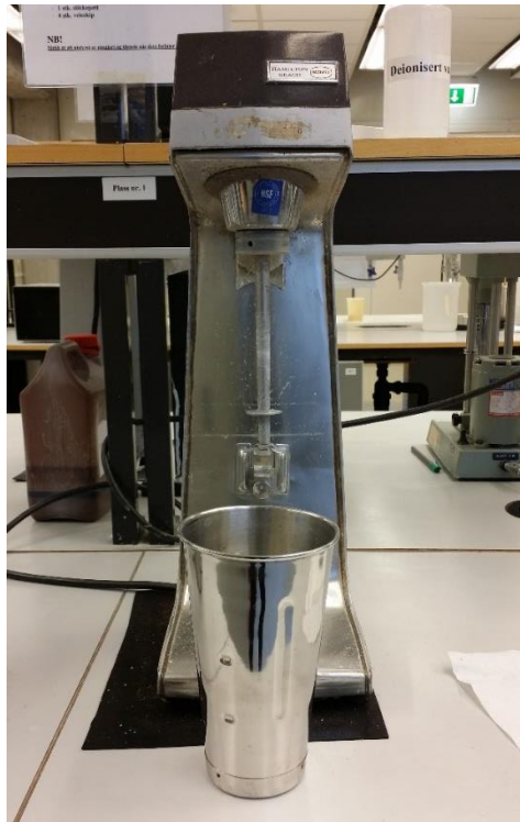
Figure 3-8: Hamilton Beach mixers used in the making of OBM and WBM
