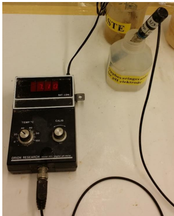
Figure 3-20: Orion Research digital pH meter
