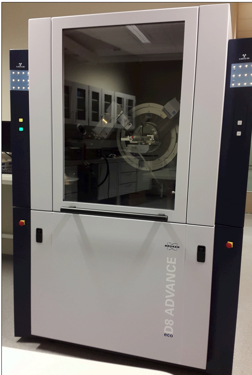
Figure 2.12: Bruker D8 Advance ECO XRD located at UiS.
