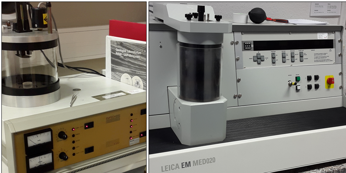
Figure 2.3: Carbon coating machines: Emitech K550 Sputter Coater used for coating the mounds with carbon before FE-SEM analyses, and Leica EM MED020 used for coating the mounds with carbon before analyses with MLA and EMPA.
