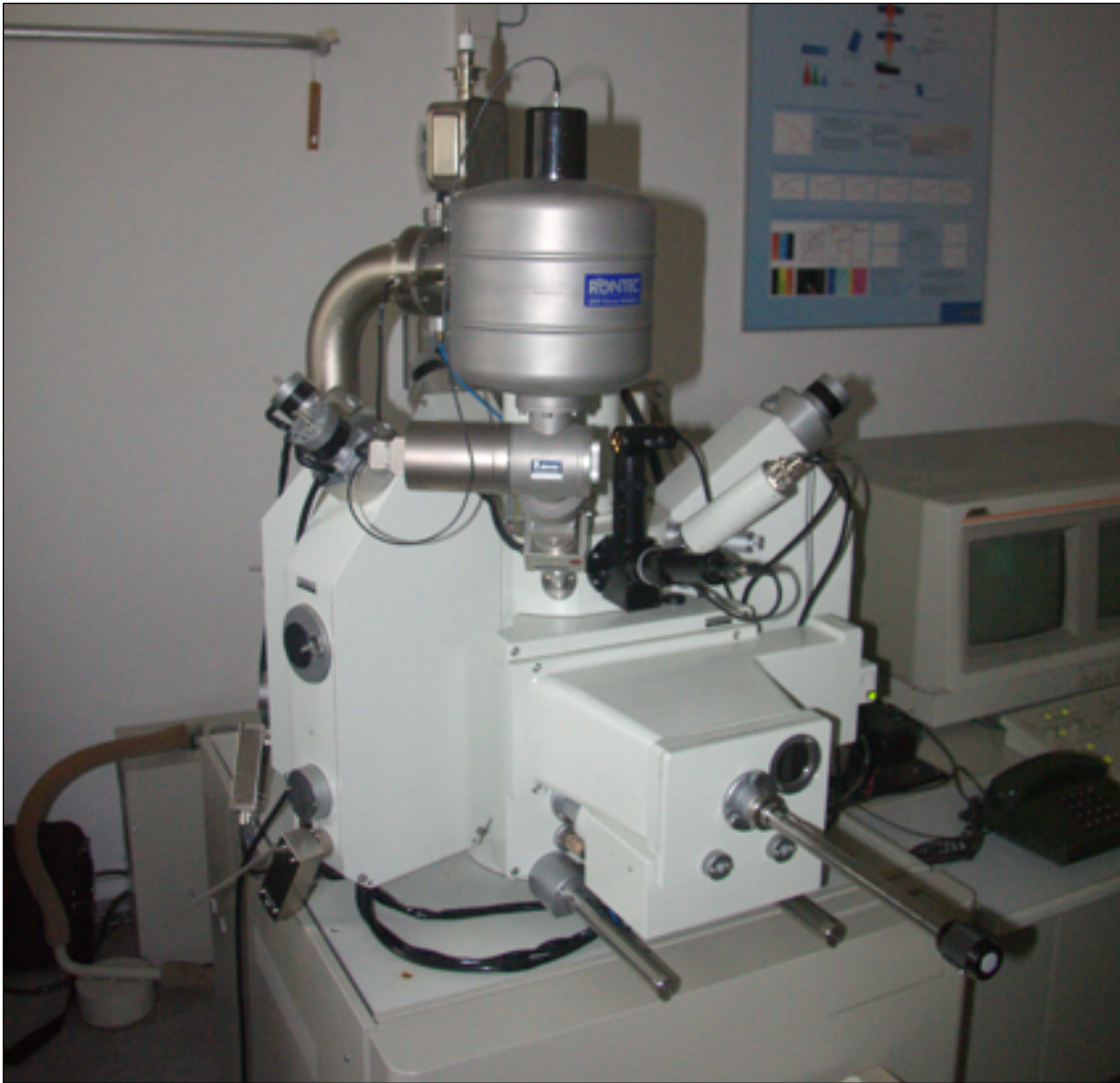
Figure 2.15: JEOL microprobe JXA 8900 located at TU Bergakademie Freiberg (photo by Sabine Haser).
