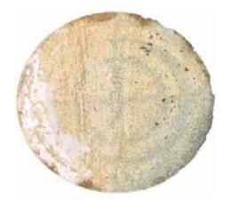
Fig. 6. A picture showing filter cake (white substance) formed at the core inlet during injection of 0.5 wt.% colloid solution containing 0.08 µm size particles into Kirby sandstone core. The narrow pore channels in Kirby core prevented some of the particles from penetrating the inlet of the core.
