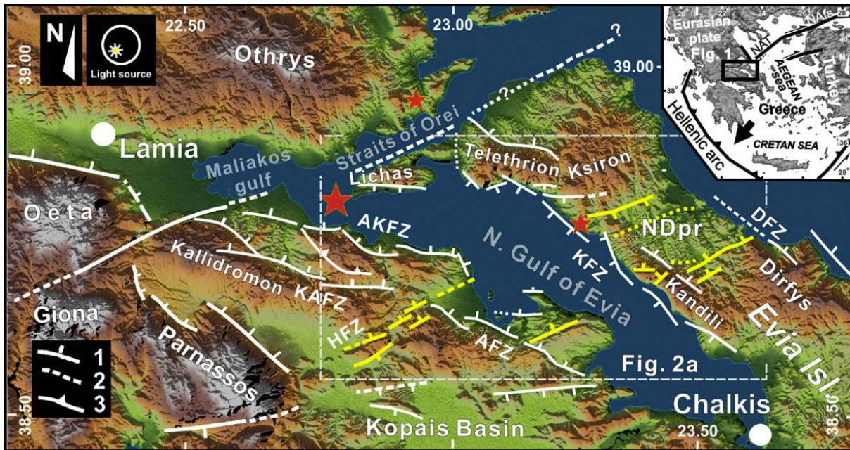
Figure 24 Map of Northern Gulf of Evia and surrounded the area with suggested transverse faults in yellow lines, NDpr: Nileas depression and KAFZ: Kallidromon f.z., 1: (oblique) normal faults, 2: probable f.z. Traces, 3: apparently reverse fault (rotated normal fault) Palyvos et al. (2006).
