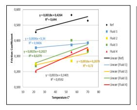
**Figure 5**: MoS<sub>2</sub> treated and reference drilling fluids average friction coefficients
