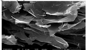
Figure 2: SEM analysis of Graphene
