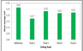
Figure 8: Average friction coefficients of the three temperatures data
