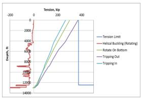
**Figure 11:** Maximum length drilling with the reference fluid without exceeding the tensile limit
