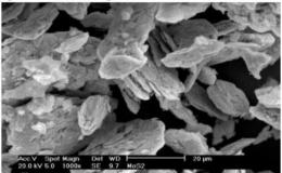
Figure 1: SEM analysis of MoS<sub>2</sub> particles
