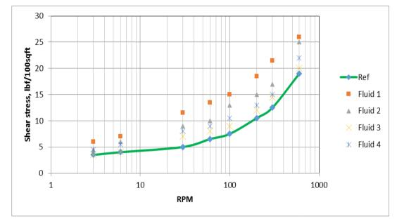
Figure 3: Viscometer measurement of test matrix – Table 1.- MoS2
