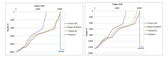
**Figure 9**: Maximum length drilling with the reference fluid without exceeding the torque limit
