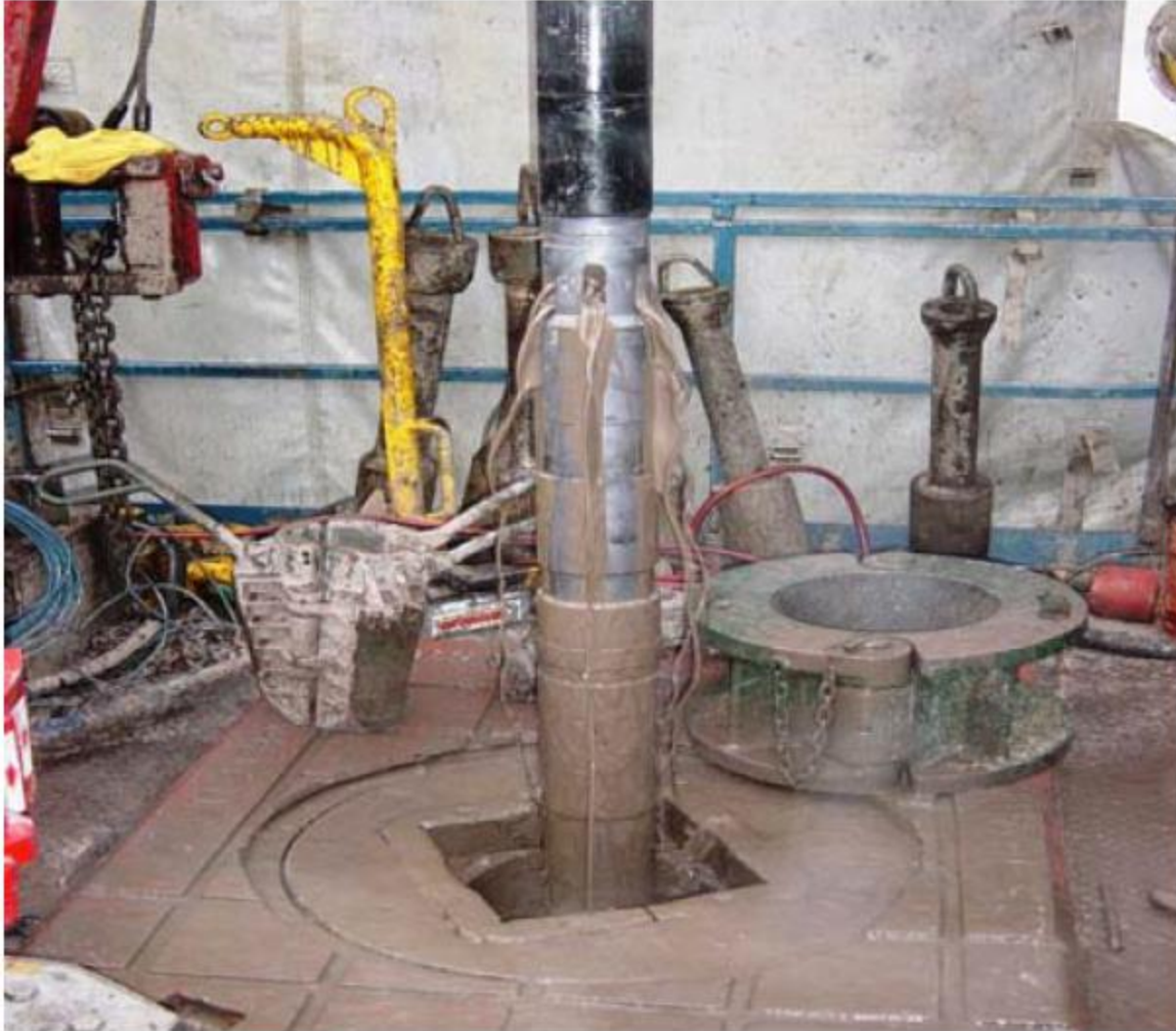
Figure 8 - Inner annulus tool on field trial, which is run inside casing (Howlett, et al., 2006)
