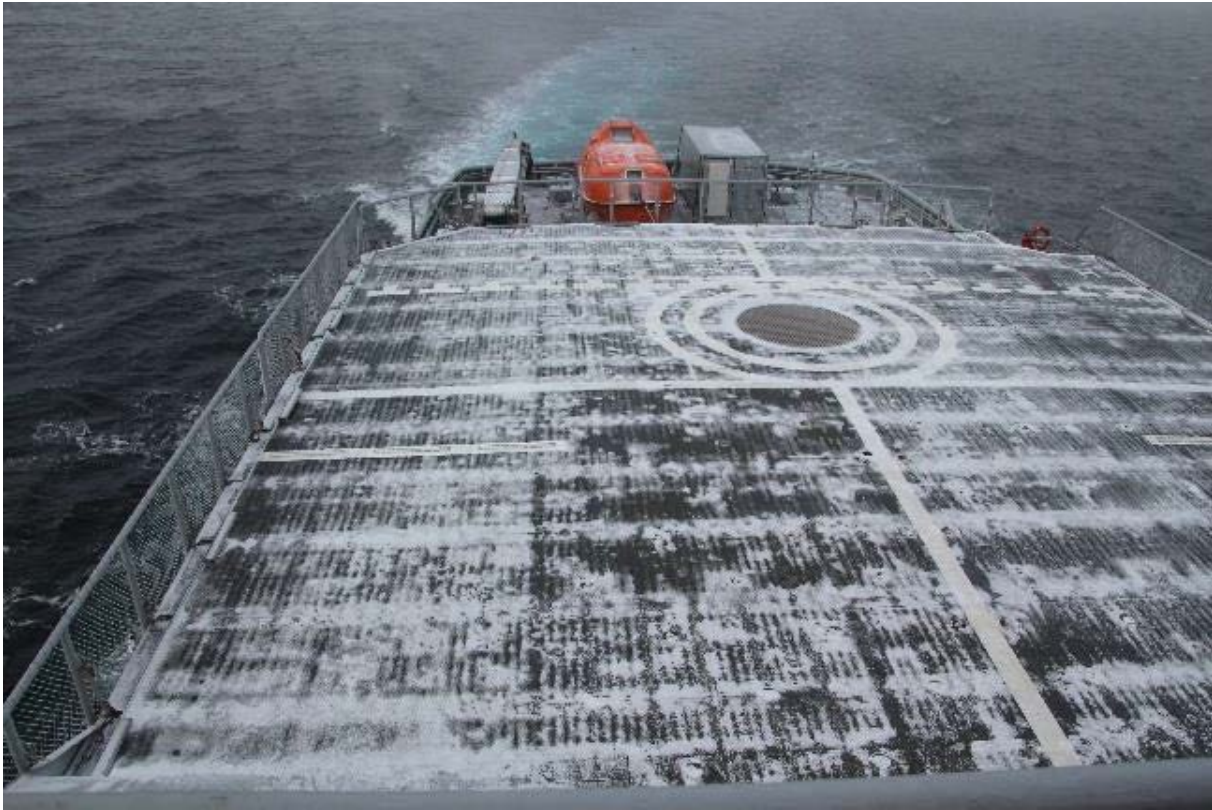
Figure 37: Snow accumulation on heli-deck of KV Svalbard during 2016 exercise @Trond Spande
