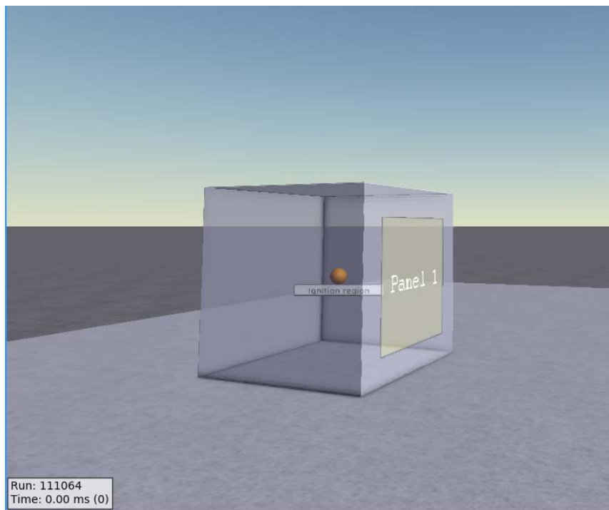
Figure 6. Simulation 3D plot, central ignition and 125 m 3 of an enclosure with pressure relief panel (1/2 of the front wall area)
