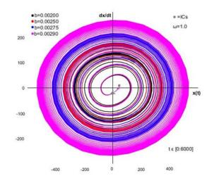
Figure 12: As b increases, the stiffness of the structure decreases, allowing more movement of the structure. This results in larger amplitude limit cycles.
