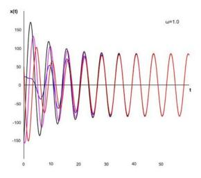
**Figure 2:** Phase plane diagram for a system with nonlinear drag force at resonance,  $\omega=1$ , Four different trajectories (with different initial conditions, IC) are shown, which all spiral towards the limit cycle marked in red.
