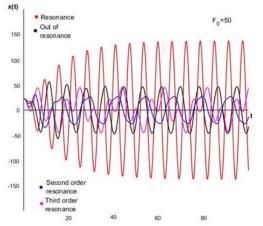
**Figure 13:** Systems with different degree of resonance subjected to loading from Equation (6) in the phase plane.
