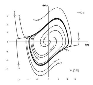
Figure 1: Phase plane diagram for the unforced van der Pol equation exhibiting a clear limit cycle.
