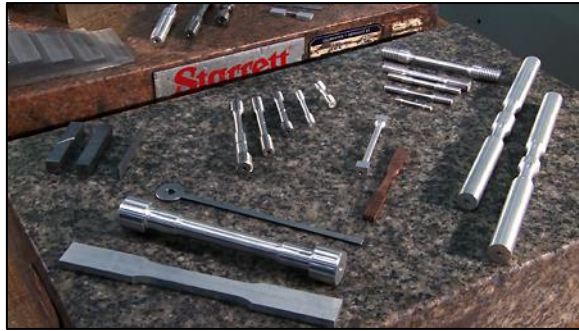
Figure 2-11: Types of shaft/pipe specimen [Laboratory Testing Inc.]
