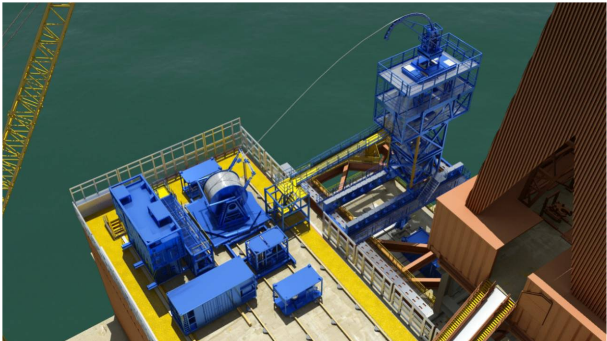
Figure 2.3: Coiled Tubing setup (Paaske 2017).
