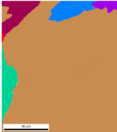
Figure 4-28 A sample from the YZ plane. A grain almost take up the whole sample size.
