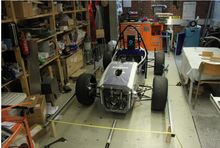
Figure 3.1: The measurement rig used to measure toe in roll and heave. The steel beams are mounted to the wheels with a rod through the hub, and supported at wheel center and parallel to the floor by the wooden blocks at each end.
