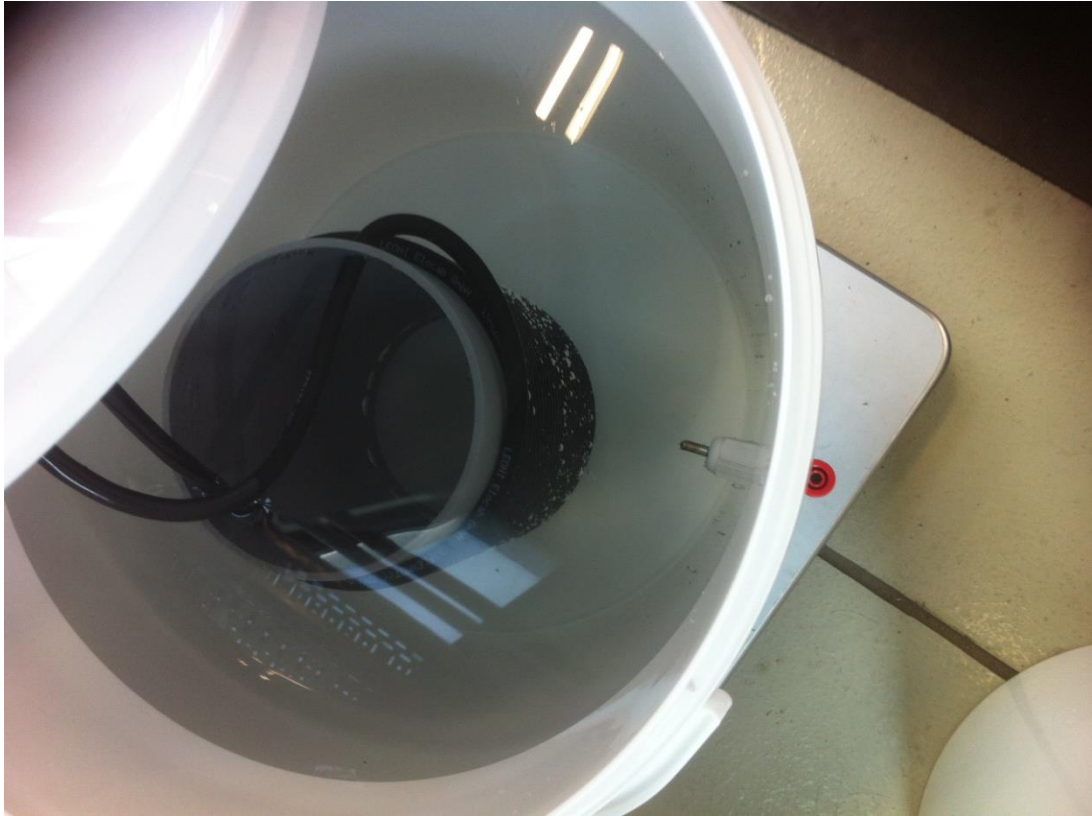
Figure 39 cable 2 coiled on PP pipe with inner diameter 100 mm
