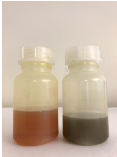
Figure 7.1: Fresh new oil (left) vs. contaminated oil (right) from the thruster pedestal.
