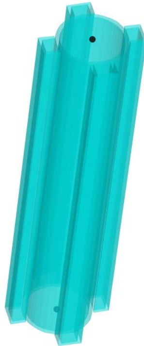
Figure 6.28: 3D view of the channel section in both directions attached to the tubular member
