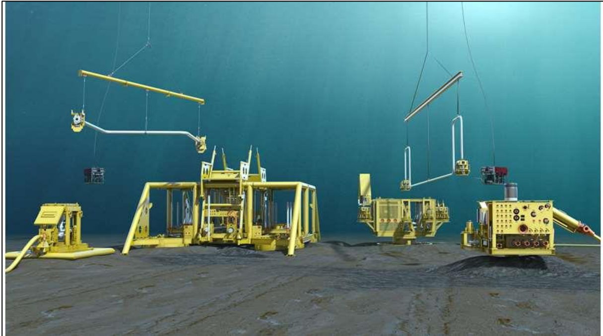
Figure 2-1: Installing subsea production systems (Aker Solutions, n.a.)
