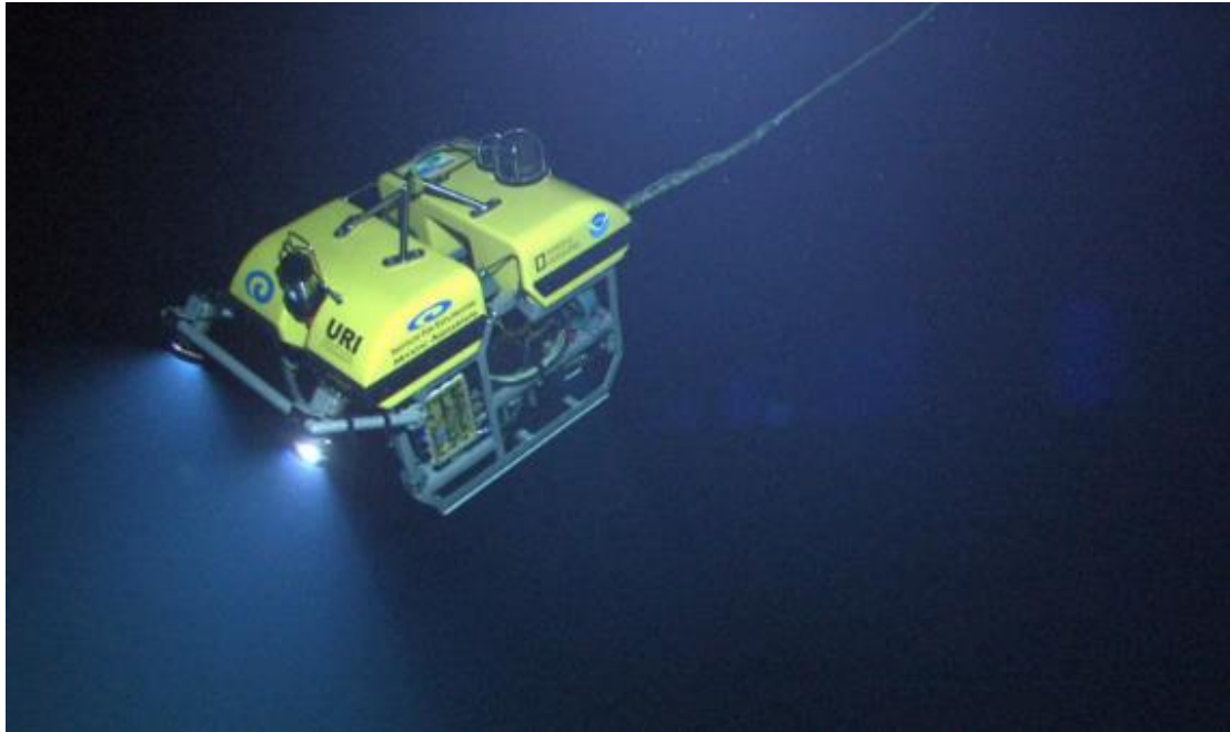
Figure 25 an underwater ROV(Pirpir5, 2014)
