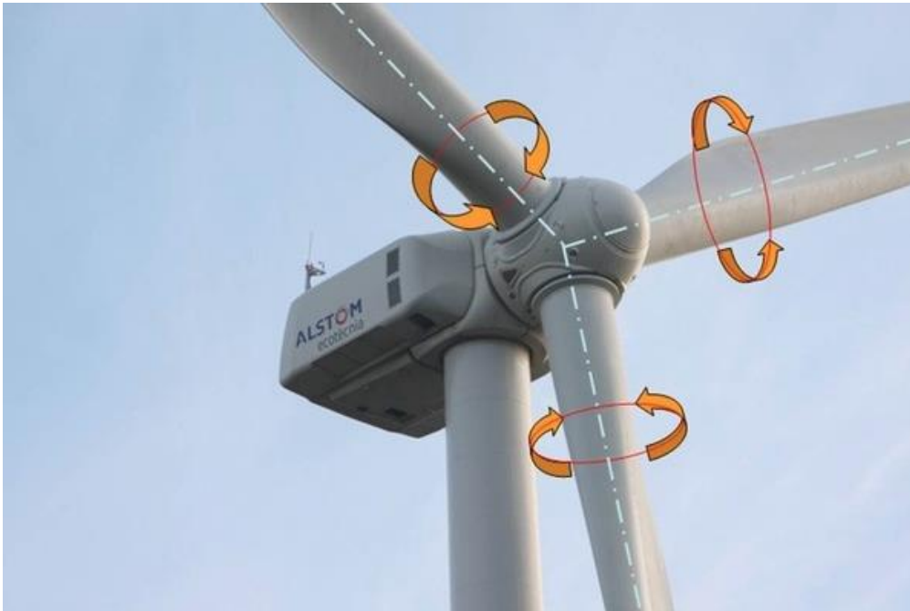
Figure 22 pitch control by rotating blades (Barnard, 2018)
