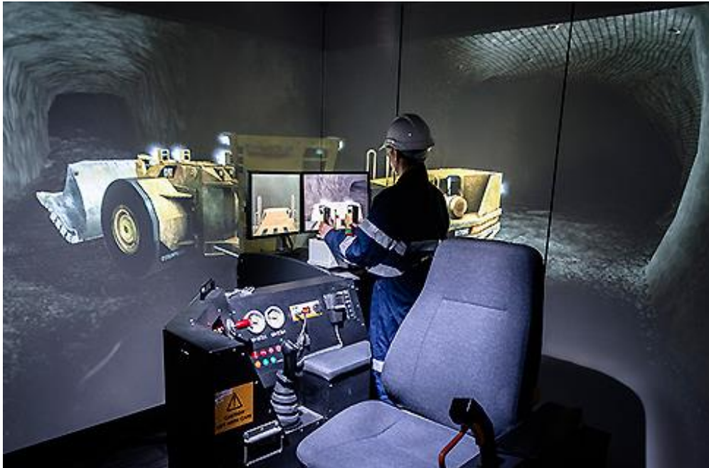
Figure 27 Remotely controlled operations (Immersive-Technologies, 2018)
