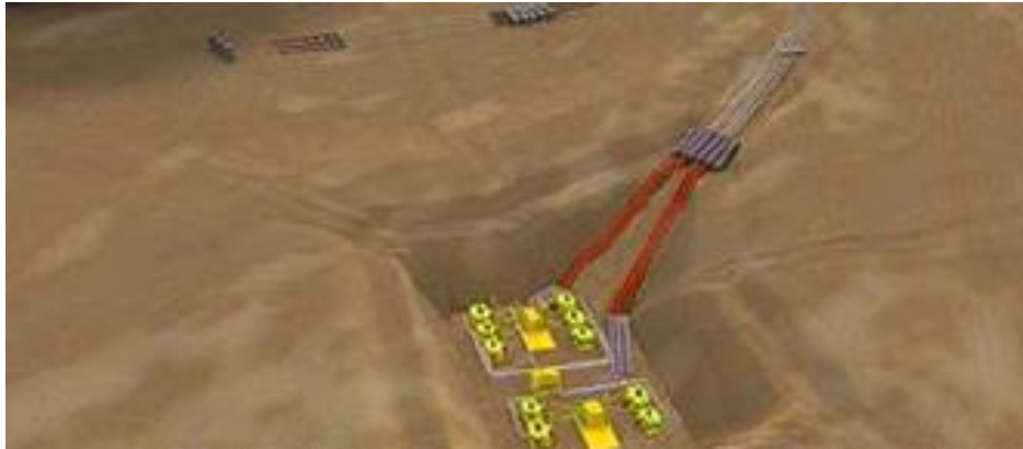
Figure 29: Subsea equipment and pipeline burial in the sea bottom (National Petroleum Council, 2015)
