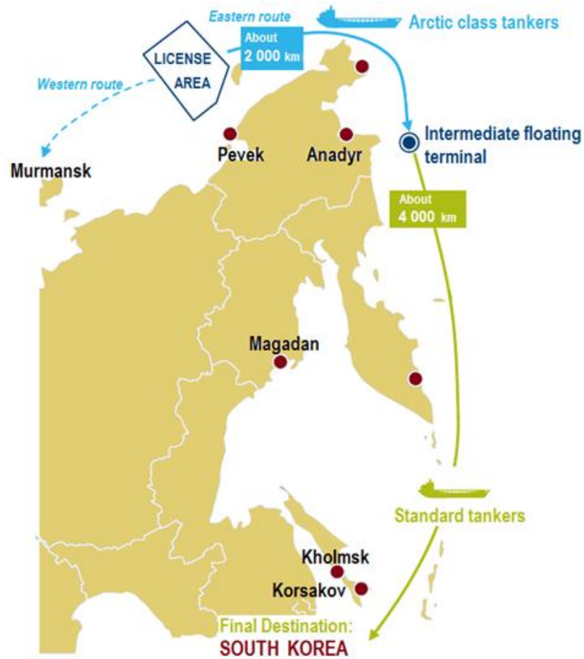
Figure 30: Concept of oil transportation by the Eastern route
