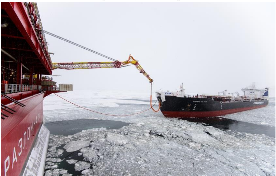
Figure 31: Direct oil offloading on the example of IRGBS Prirazlomnaya
