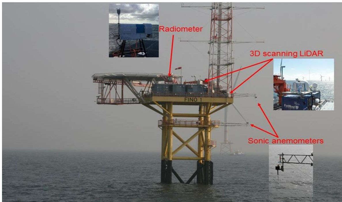
Figure 4.7 NORCOWE OBLEX-F1 Campaign Instruments (Flügge, 2018).
