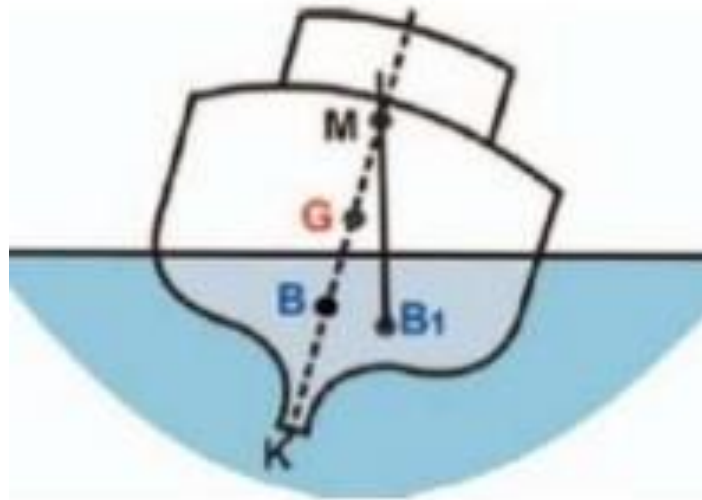
Figure 8.2 Metacentric height ( www.slideshare.net )
