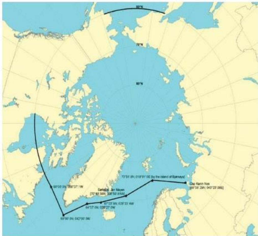
Figure 10.3.1 The Arctic water area, which is subject to the requirements of the Polar Code ( www.imo.org )
