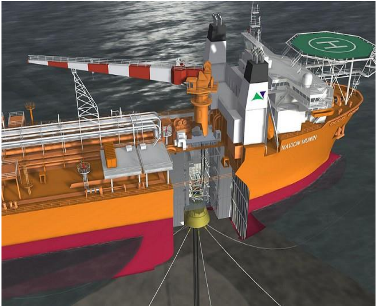
Figure 9.2.1 Double positioning system (Khairov, 2016)
