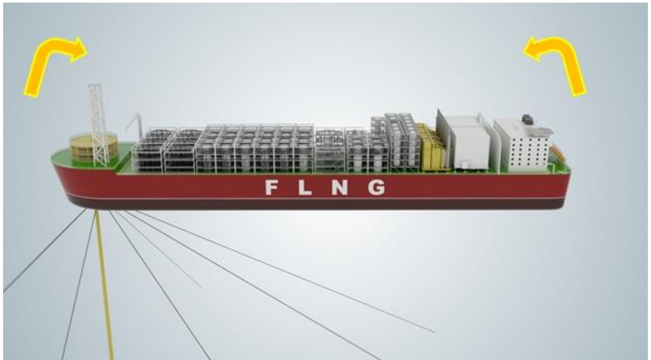
Figure 8.5 Pitch motion of the vessel ( www.seafasten.com )
