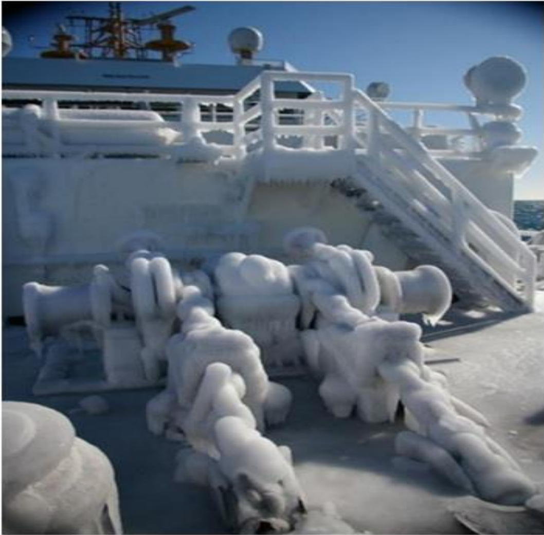
Figure 10.1 Icing on a vessel ( www.arctic-operations-handbook.info )
