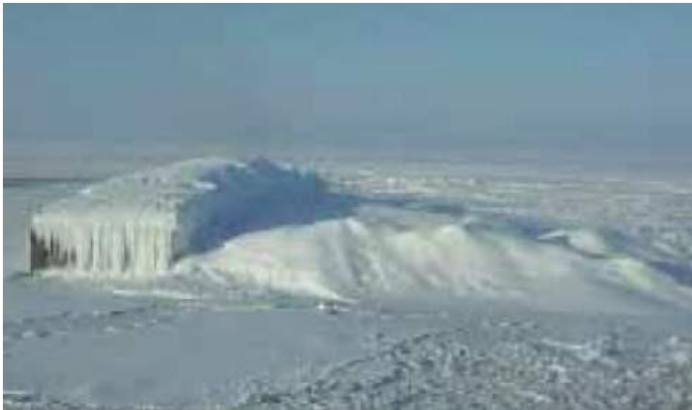
Figure 5.13: Grounded barge in the North Caspian Sea (Bastian et al., 2004).
