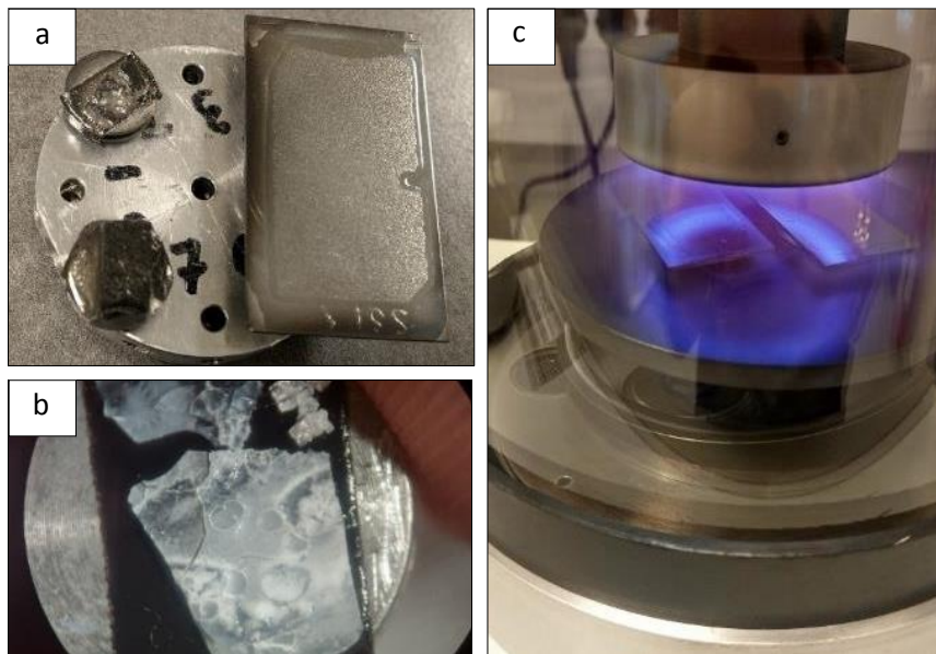
Figure 13. Sample preparation for SEM and EDS. a) A sample holder containing 3 samples: dried SS (upper left corner), core fragment (lower left corner) and thin section (right side). b) A close-up of the mounted dried SS + HCl + DW. c) Pd coating.
