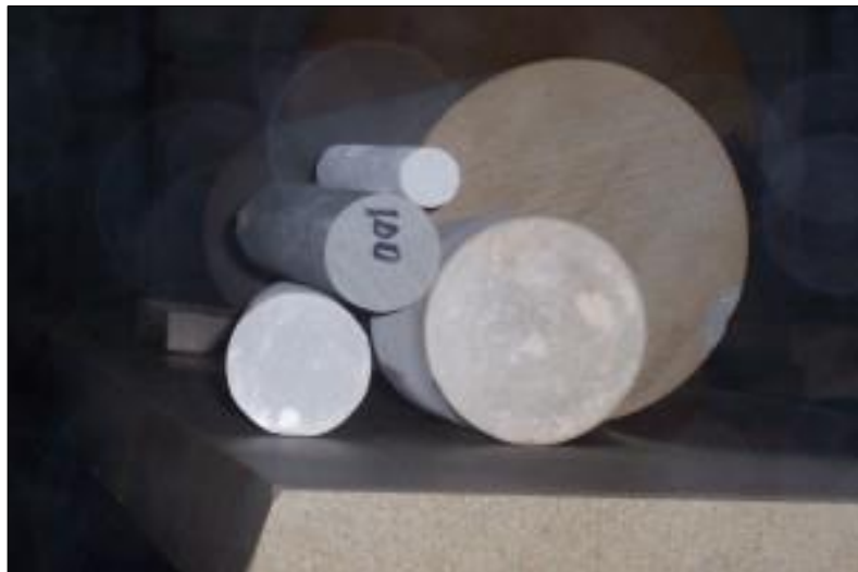
Figure 4. Berea Sandstone cores in a variety of diameters, permeabilities and porosities (ClevelandQuarries, 2018).
