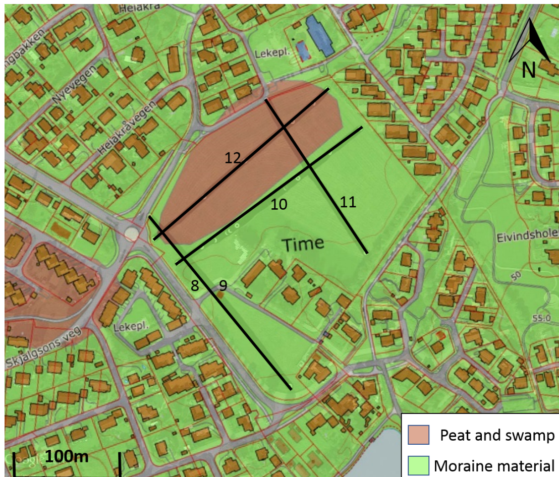
Figure 16: Geology of Bryne site, with acquired GPR lines marked.
