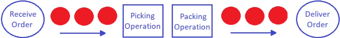
Figure 4. 12 – Waiting line model when the picking and packing is performed by the same person.
