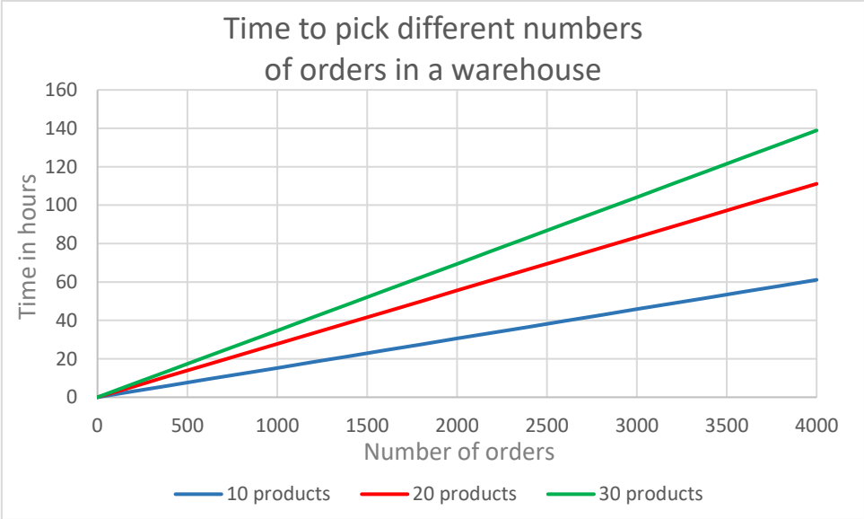
Figure 4. 7 – The total time of picking different numbers of orders in a warehouse-based model for orders with an average of 10, 20, and 30 products per order
