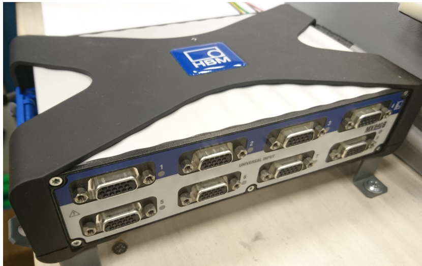
Figure 2.9: 8-channel HBM QuantumX MX840B
