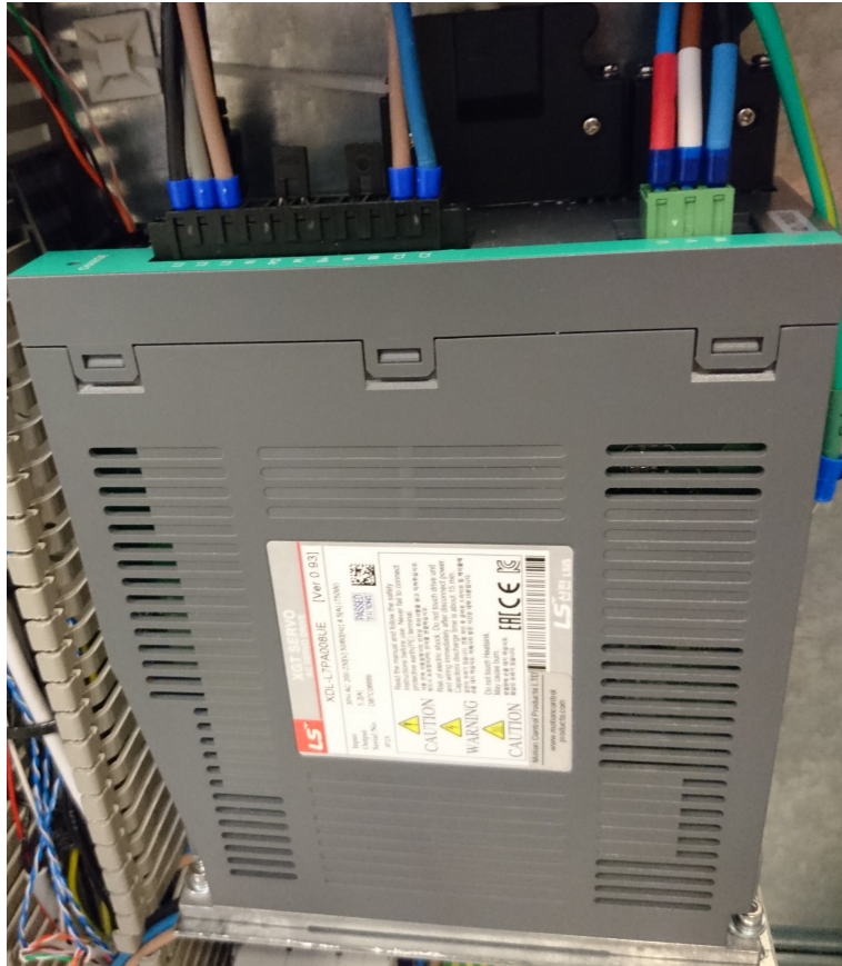
Figure 2.5: Top drive driver, XDL-L7PA008UE from LS industrial systems.
