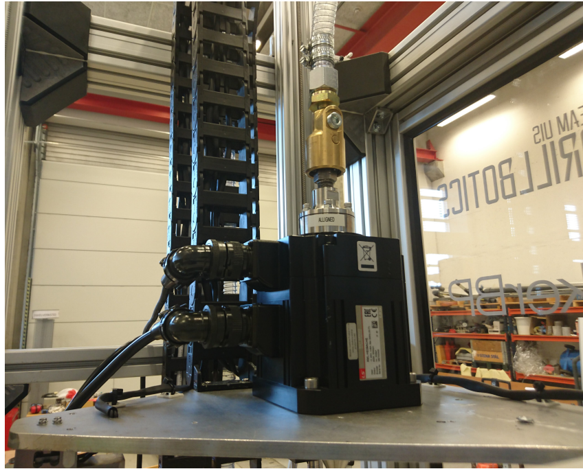
Figure 2.4: Top drive of the laboratory rig.
