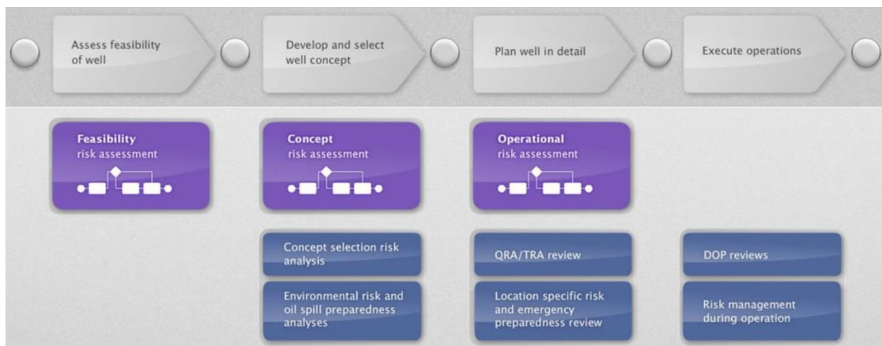
Figure 5: Summary of DW600: Construction of Development Wells. The four main phases are feasibility, concept selection, detailed planning and execution. First three phases include risk assessments (purple boxes). Blue boxes are additional RM activities but which are not covered in this work. From: (Statoil et al., 2013)
