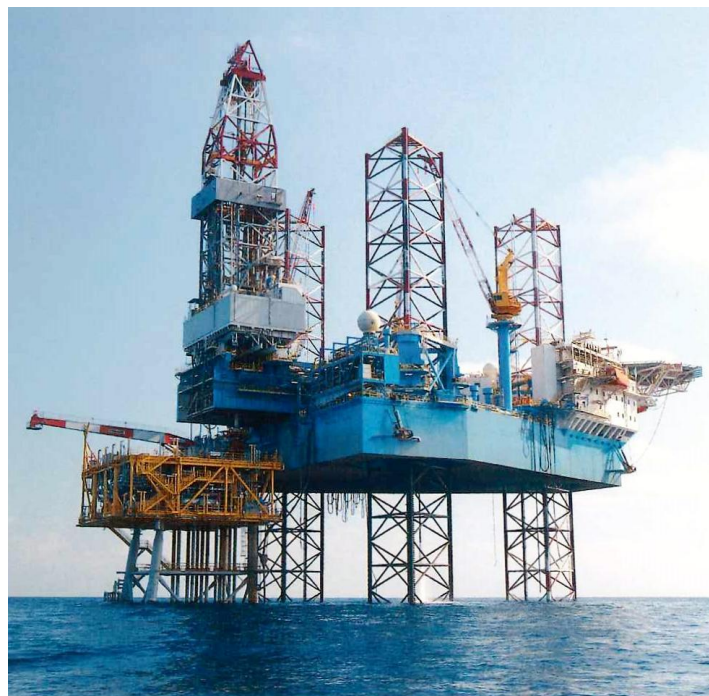
Figure 6: Jack-up rig with derrick cantilevered over a wellhead platform [16]
