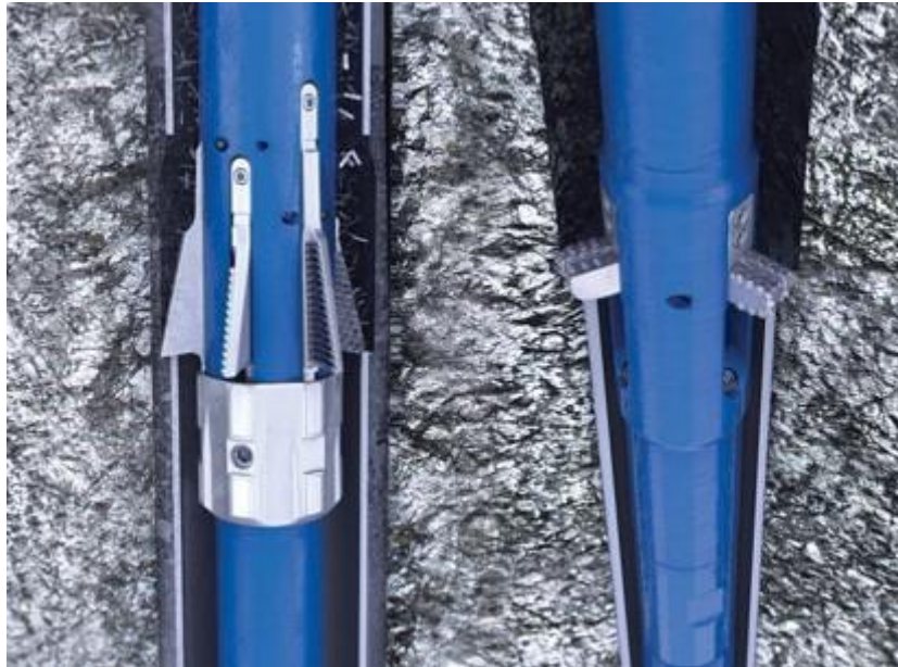
Figure 8: Section milling (left), where cement and casing are ground away by hydraulic extended blades. Underreaming (right) grinds away more formation to expose fresh formation for better cement bonding [18]
