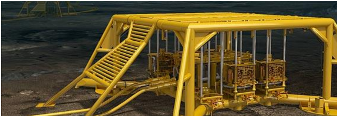
Figure 53: Subsea template with protective structure [191]
