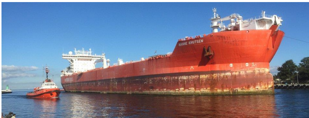
Figure 69: The Hanne Knutsen, which has been converted to an FSO for the Martin Linge development [207]
