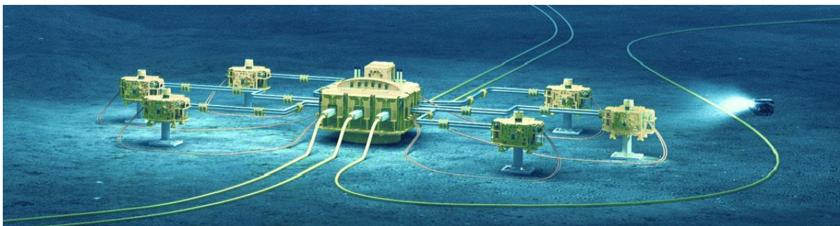
Figure 43: A number of subsea wells surrounding a central manifold [113]
