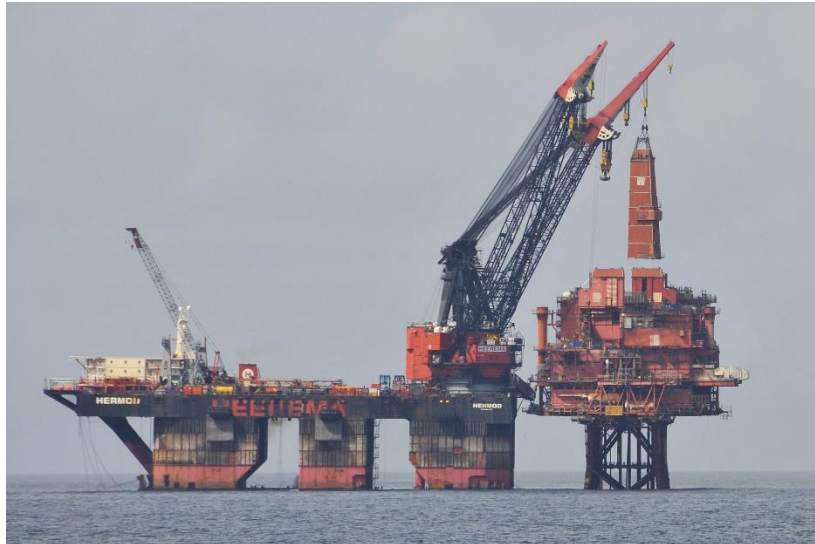
Figure 10: HMC Hermod removing a derrick from North-West Hutton [22]
