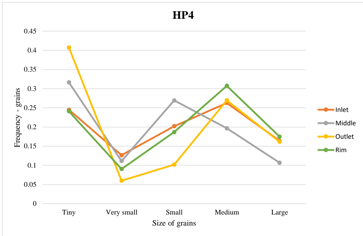
Figure 4.3. 10: The frequency of the grains as a function of different grain sizes for HP4. (tiny: 0.87 \times 0.87 \mu\text{m} , very small: 0.87 \times 0.87 - 1.74 \times 1.74 \mu\text{m} , small: 1.74 \times 1.74 - 2.9 \times 2.9 \mu\text{m} , medium: 2.9 \times 2.9 - 6.38 \times 6.38 \mu\text{m} , large: 6.38 \times 6.38 \mu\text{m} )
