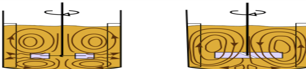
Figure 25: Radial flow pattern (left) and axial flow pattern (right) [28].
