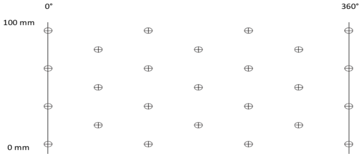
Figure 11: Showing a 100 mm long illustration of the casing with 60 degrees phasing's
