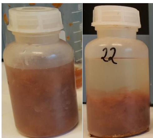
Figure 36: Samples before and after centrifuge, treated with chemicals
