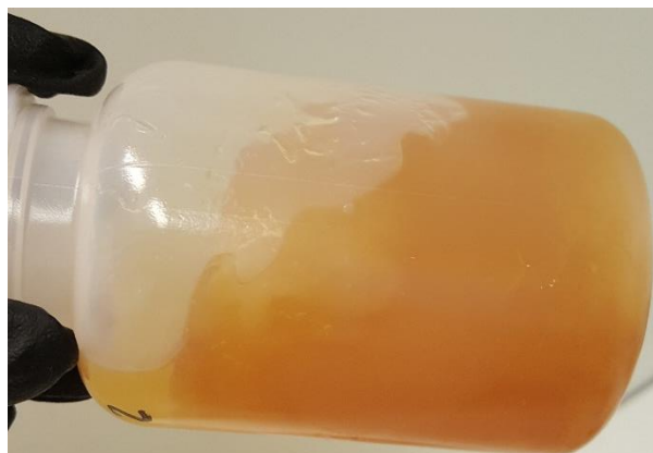
Figure 33: Sample of XG treated with coagulants and centrifuge
