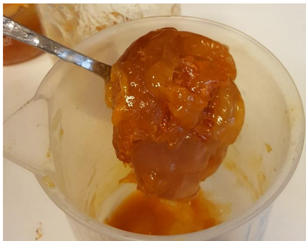
Figure 37: A strong, hard and big floc of chemical treated XG solution.
