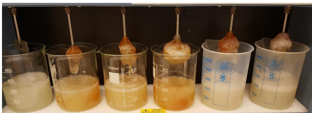
Figure 32: XG flocculated around jar tester paddles
