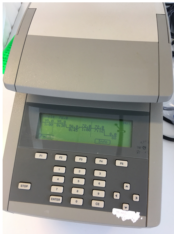
Figure 9: Thermal cycler showing PCR program.
