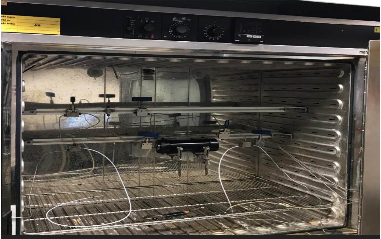
Figure 71 The Setup for core flooding at IRIS
