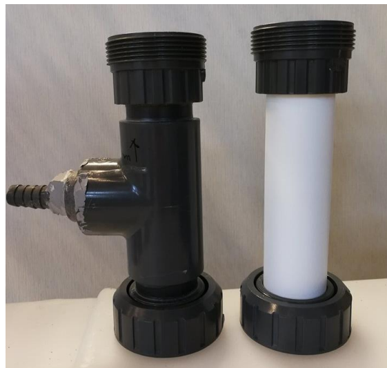
Figure 35 Replacing three-way pipe
