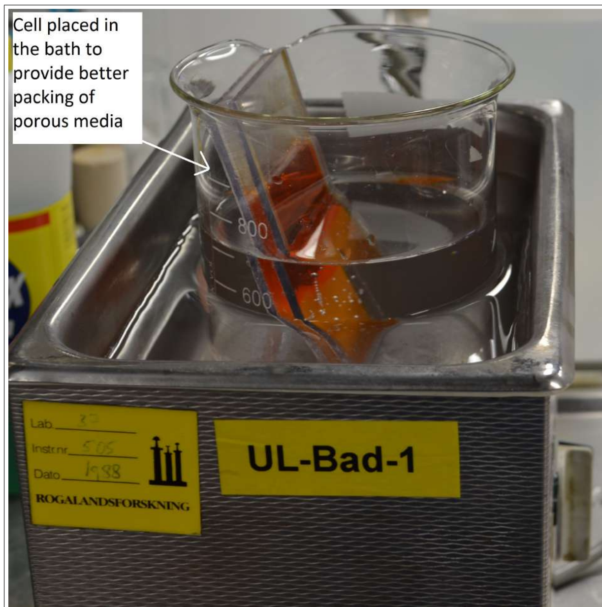
Figure 4.7: Polycarbonate cell in an ultrasonic bath.
