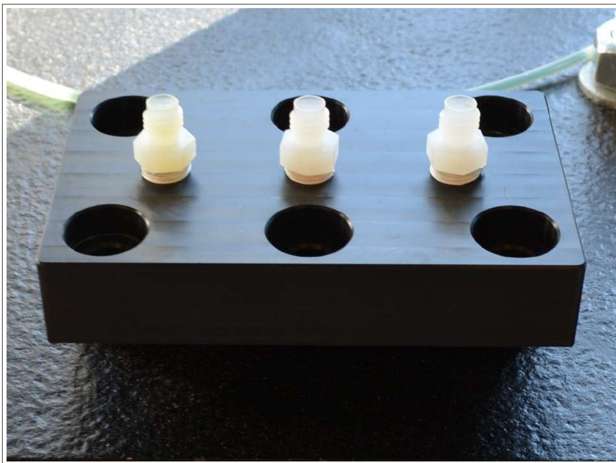
Figure 4.9: Filter module used in the POM cell.
