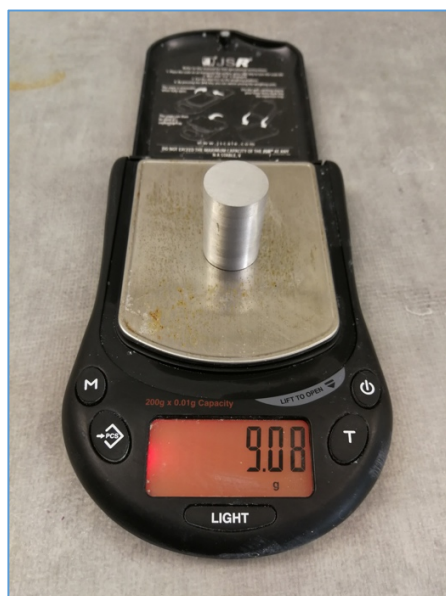
Figure 3-5: Weighing scale to measure cylindrical sample mass
