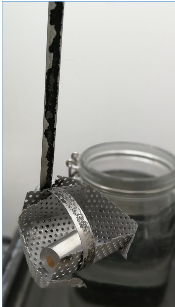
Figure 4-10: Perforated sample holder to ensure uniform exposure of sample's surface area to test fluid
