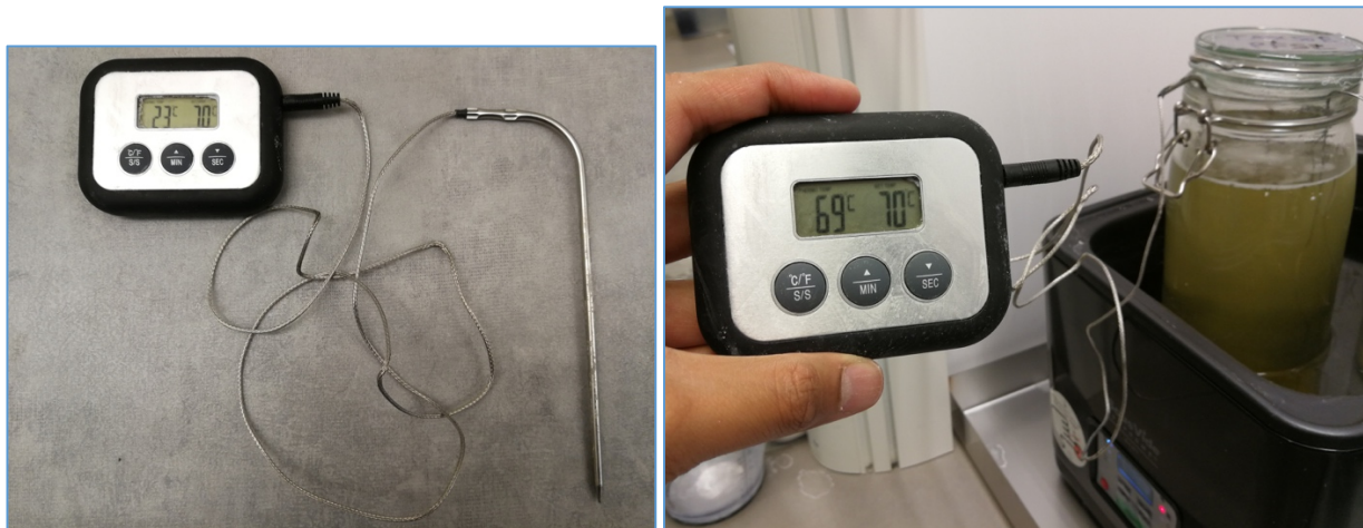
Figure 3-4: Thermostat used to monitor temperature of test fluid
