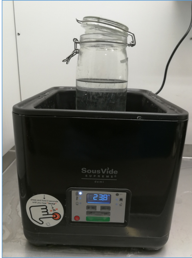
Figure 3-3: Heater used to heat and maintain a water bath at required temperature
