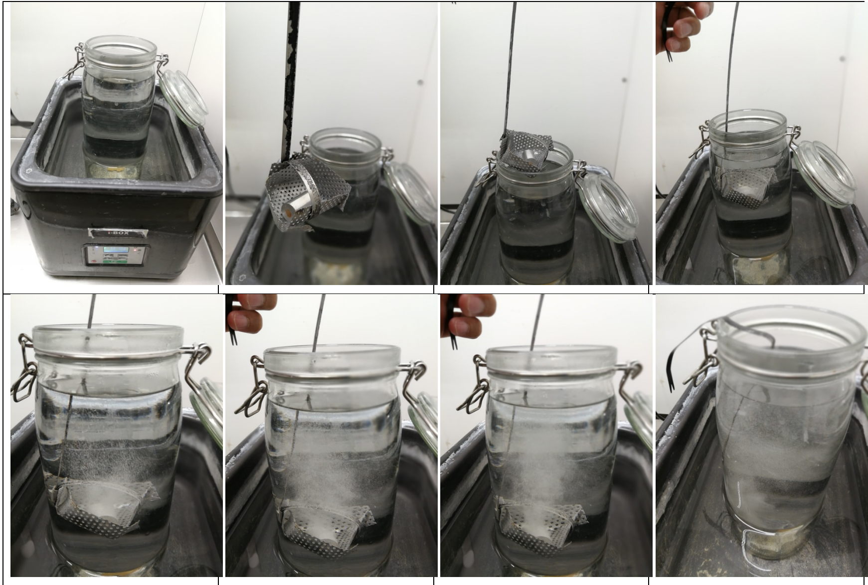
Figure 3-11: Lowering the dissolvable material sample into the test fluid using sample holder
