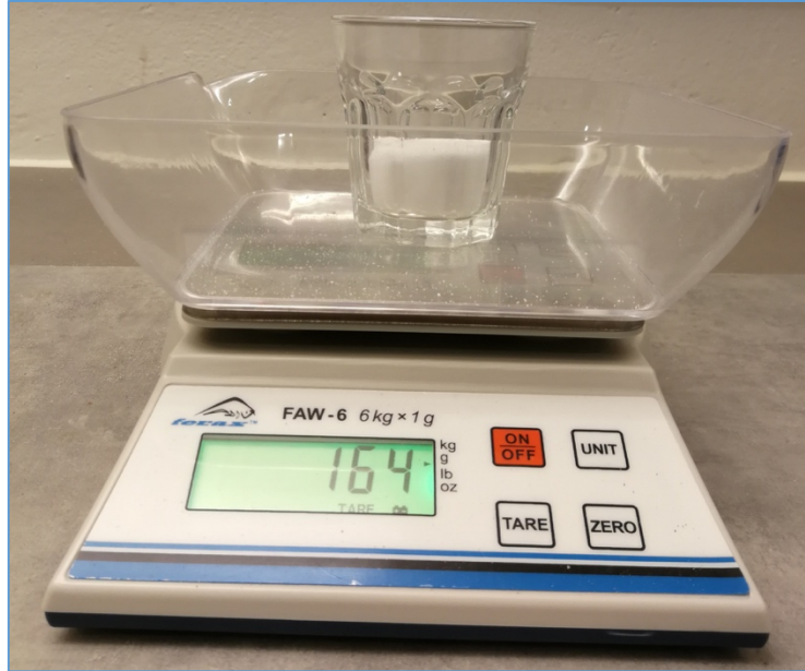
Figure 3-6: Scale used to weigh NaCl crystals for test fluid preparation
