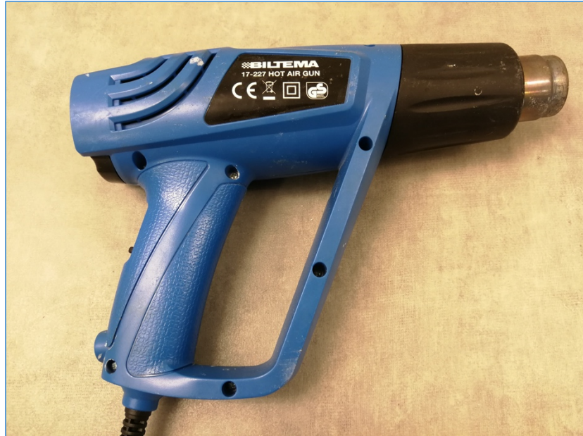
Figure 3-8: Heat Gun used to dry samples
