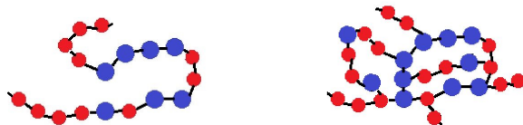
Figure 3: Symbolic representations of linear (left fig.) and cross linked molecule structure (right fig.)
