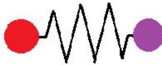
Figure 18: polymer molecule in Hookean dumbbell model
