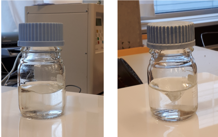
Figure 7: The beaker with magnet inside is set into magnet field. (left fig.) beaker with polymer (right fig.) beaker with water
