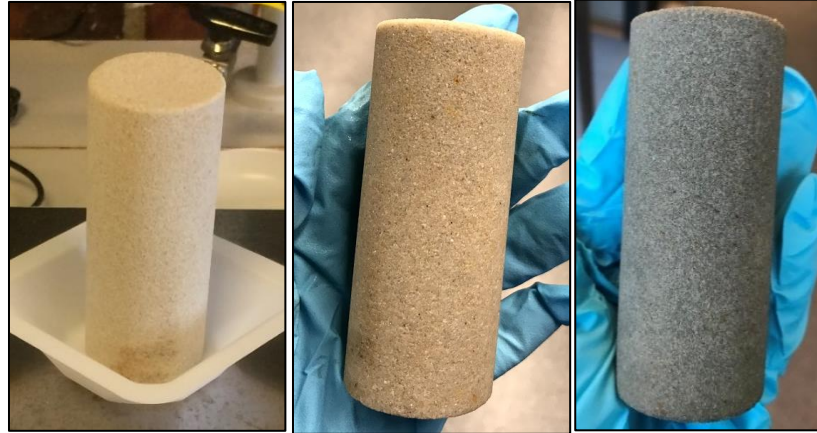
Figure 14. Conditions of OWB_3 a) before, b) after wettability alteration using Quilon L solution (3% wt) and c) after temperature aging at 95° in the oven.
