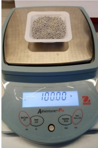
Figure C - 6: Weighing scales –weight of the particles
