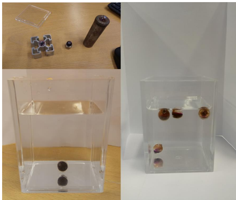
Figure C - 3: Design and test of the “Neutral glass particles”
