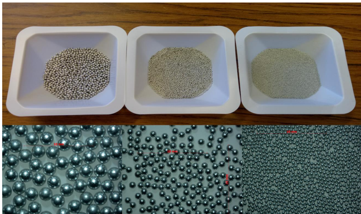
Figure C - 5: Aluminum spherical particles. Front left to right: 2 mm, 1 mm and 0.5 mm mean diameter.
