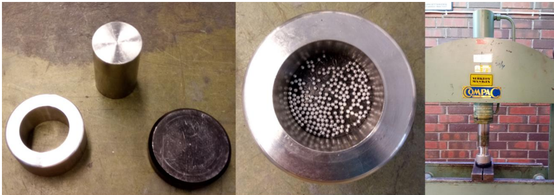
Figure C - 7: Tools and equipment to make flat particles
