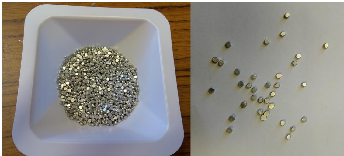
Figure C - 8: Homemade Aluminum flat particles
