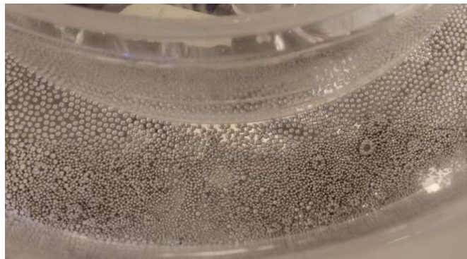
Figure 6: Particles agglomeration in the annular channel
