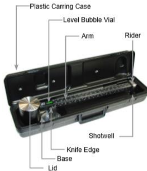
Figure 2.2. Metal mud balance complete with carrying case [5]
